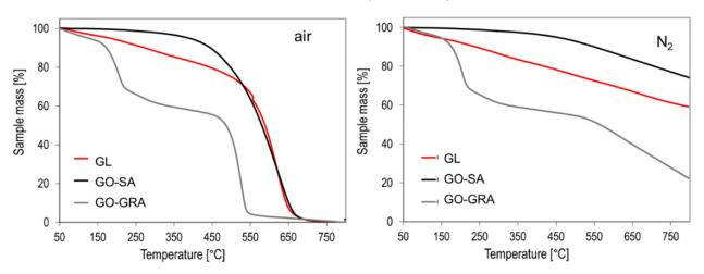
(around 500 °C) with respect to GL and GO-SA materials, testifying the presence of a more defective surface, with sites easily attacked by  $O_2$  [77].
