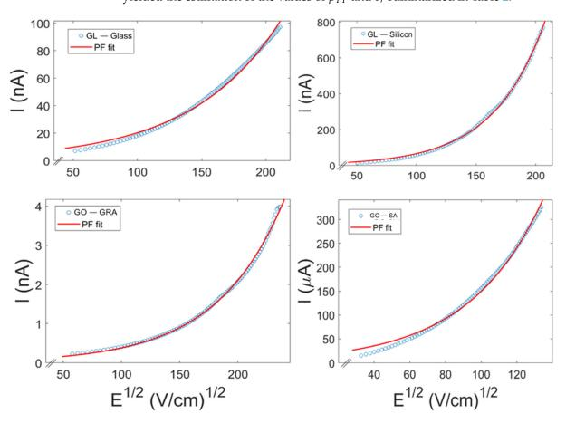
**Figure 11.** Plots of I vs  $E^{1/2}$ , where E is the electric field. The curves are fitted by Poole–Frenkel (PF) model.
