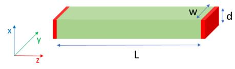
**Figure 10.** Sketch of the device as a plane parallel plate capacitor (in red) filled with a material (GRMs) with dielectric constant  $\epsilon_r$  (in green).
