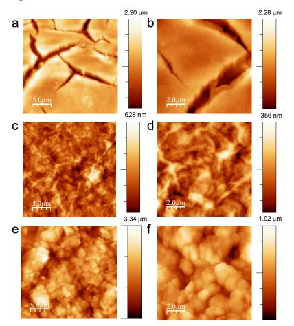
**Figure 4.** Non-contact-mode AFM images ((**a**,**c**,**e**): 25  $\mu$ m × 25  $\mu$ m and (**b**,**d**,**f**): 10  $\mu$ m × 10  $\mu$ m) on: GL film (**a**,**b**); GO-GRA film (**c**,**d**); GO-SA film (**e**,**f**).
