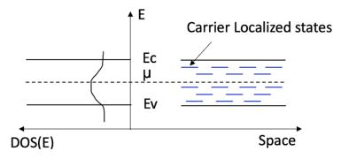
**Figure 8.** Sketch of the band diagrams and density of states as a function of energy for an amorphous material. Ec, Ev,  $\mu$  and DOS(E) represent: conduction band energy, valence band energy, chemical potential and the density of the state, respectively.
