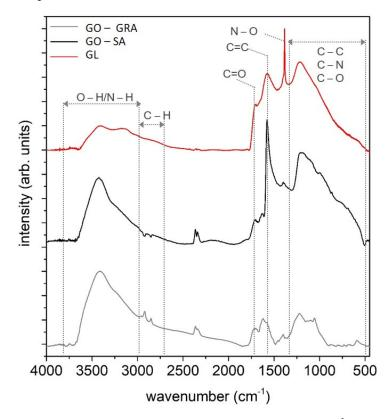
**Figure 3.** FTIR spectra of the three GRMs in the  $450-4000 \text{ cm}^{-1}$  region.
