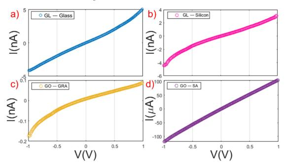
**Figure 6.** IV characteristics of the four films deposited on different substrates (glass, silicon) in the  $\pm 1$  V range of the applied bias voltage. Plot (**a**) IV curve of GL film on glass; (**b**) IV curve of GL film on silicon; (**c**) IV curve of GO-GRA film on a glass substrate; (**d**) IV curve of GO-SA film on a glass substrate.
