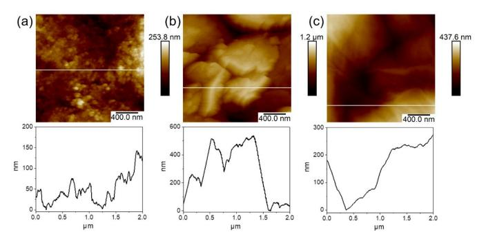
**Figure 5.** Non-contact-mode AFM images  $(2 \ \mu m \times 2 \ \mu m)$  on: (**a**) GL film; (**b**) GO-GRA film; (**c**) GO-SA film. Images show a reference line fixed at 2  $\ \mu m$  to highlight film surface roughness (lower panels).
