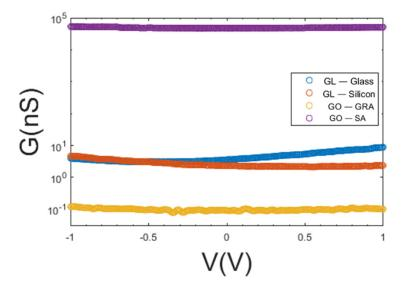
**Figure 7.** GV curves of four films deposited on different substrates: GL films on glass and Si/SiO<sub>2</sub>; GO-GRA and GO-SA films both on glass.
