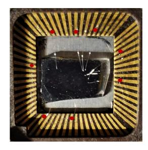
**Figure 1.** GL film on glass substrate glued onto chip carrier. All electrical connections between the sample and the chip holder (red filled circles) were made by Al wires with a bonding machine.
