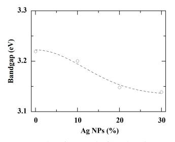
**Figure 11.** Bandgap of pure ZnO thin film and ZnO/Ag(NPs) nanocomposite thin films. The dashed curve is provided as a guide for the eye.
