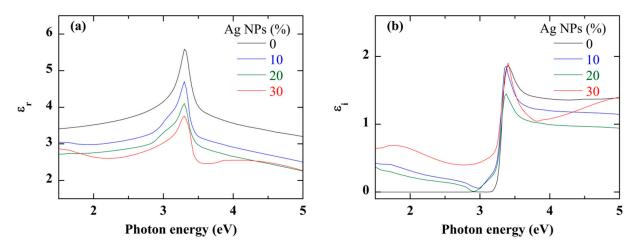
**Figure 10.** Real part (**a**) and imaginary part (**b**) of the dielectric function of the ZnO/Ag(NPs) nanocomposite film loaded with different contents of Ag NPs.
