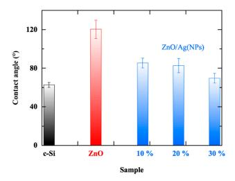
**Figure 8.** Contact angle value of c-Si substrate, ZnO thin film, and nanocomposite thin films with different Ag NPs contents.
