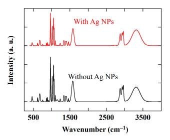
Figure 2. FTIR absorption spectrum of ZnO precursor solution without and with 10% Ag NPs.
