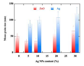
**Figure 6.** Average size of ZnO grains and Ag NPs as a function of Ag NPs content in the nanocomposite deduced from SEM images.
