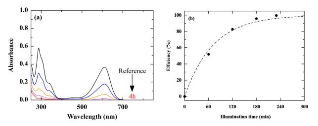
**Figure 16.** Absorbance spectrum (**a**) and photodegradation efficiency (**b**), over time, of a Somme waterbased IC solution under solar irradiation and in the presence of a ZnO/Ag(10% NPs) photocatalyst.
