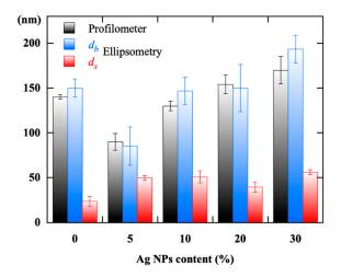
**Figure 9.** Thicknesses of the bulk layer ( $d_b$ ) and surface roughness ( $d_s$ ), determined by ellipsometry, and total thickness measured by a profilometer, of ZnO/Ag(NPs) nanocomposite films with different Ag NPs contents.
