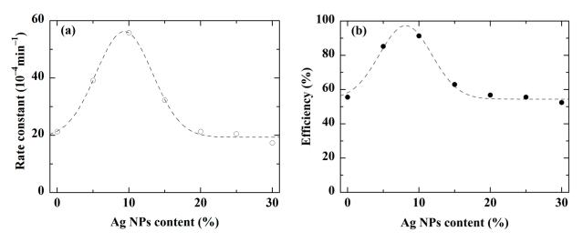
**Figure 12.** Rate constant (**a**) and photodegradation efficiency (**b**) of an IC solution after 6 h of illumination under UV irradiation, with a ZnO thin film and a ZnO/Ag(NPs) thin film loaded at different Ag(NPs) contents. The curves are provided as guides for the eye.
