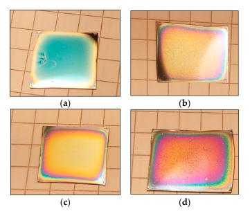
**Figure 4.** Surface appearance of ZnO/Ag(NPs) nanocomposite thin films deposited on a c-Si substrate, with a size of about  $20 \times 20 \text{ mm}^2$  and prepared with different Ag NPs contents: 0% (**a**), 5% (**b**), 10% (**c**), and 30% (**d**).
