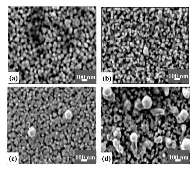
**Figure 5.** SEM images of the surface morphology, at a scale of a few hundred nm, of pure ZnO thin film (**a**) and ZnO/Ag(NPs) nanocomposite thin films elaborated with different Ag NPs: contents: 5% (**b**), 10% (**c**), and 30% (**d**).
