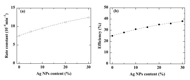
**Figure 13.** Rate constant (a) and photodegradation efficiency (b) of an IC solution after 6 h of illumination under halogen lamp irradiation equipped with a UV filter, with a ZnO thin film and a ZnO/Ag(NPs) thin film loaded at different Ag(NPs) contents. The curves are provided as guides for the eye.
