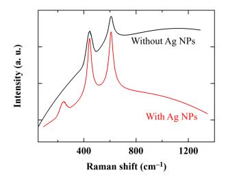
Figure 3. Raman spectrum of the ZnO precursor solution, without and with 10% Ag NPs.
