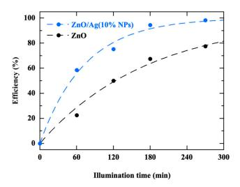
**Figure 15.** Photodegradation efficiency, over time, of an IC solution under solar irradiation by a ZnO/Ag(10% NPs) thin film and by a pure ZnO film. The curves are provided as guides for the eye.
