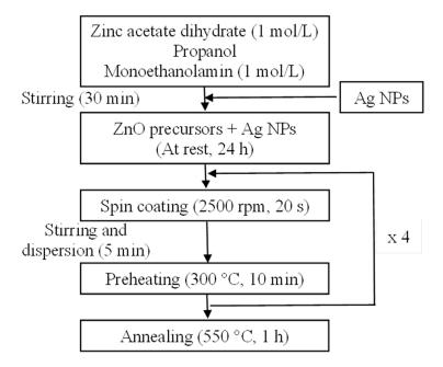
**Figure 1.** Sol–gel and spin-coating processing of ZnO nanocomposite films loaded with Ag NPs (ZnO/Ag(NPs)).
