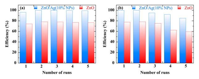
**Figure 17.** Photodegradation efficiency by a ZnO/Ag(10% NPs) photocatalyst under solar illumination of an IC solution prepared with deionized water (**a**) and Somme water (**b**), during 5 cycles of 4 h.
