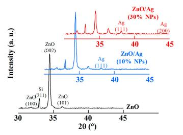
**Figure 7.** XRD diagram of pure ZnO and ZnO/Ag(NPs) nanocomposites elaborated with contents: 10% and 30% of Ag NPs.
