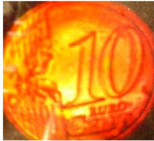
**Figure 3.** Denisyuk reflection hologram recorded in DA-based photopolymer, illuminated in white light.
