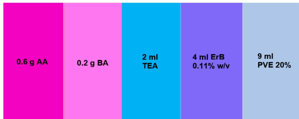
**Figure 1.** Typical chemical composition of AA-based photopolymer.
