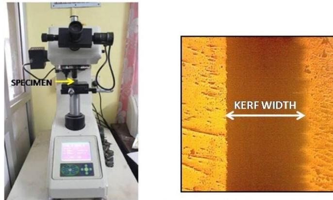
Figure 2. Measurement of Kw of machined specimen using the microscope.
