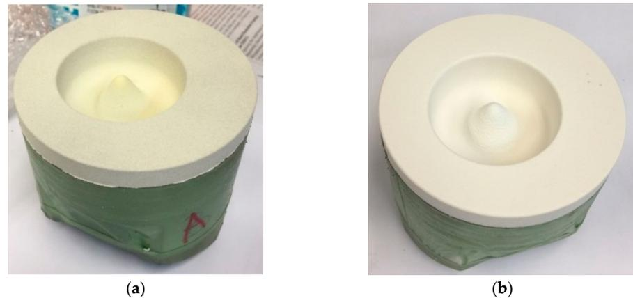
**Figure 4.** Piston coated with (a) YSZ and (b)  $\text{Al}_2\text{O}_3\cdot\text{SiO}_2$ .
