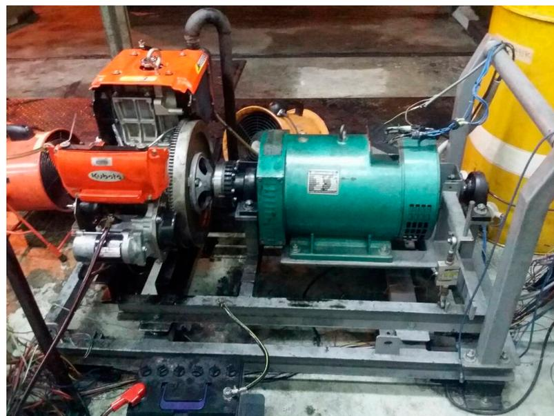
Figure 2. Kubota RT-125 diesel engine experimental setup.
