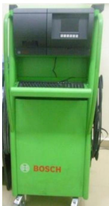
Figure 3. Photo of gas analyzer BOSCH BEA-150.
