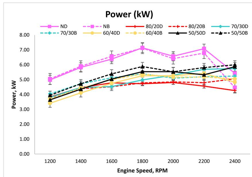
Figure 9. Power (kW) produced at various engine speed.
