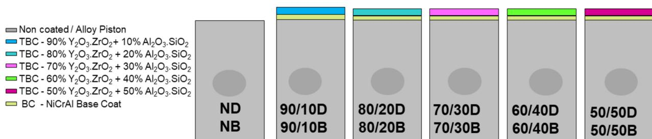
**Figure 4.** Piston crown configuration with specific coating mixture.**Table 4.** List of physical and chemical properties of biodiesel and diesel fuels.
