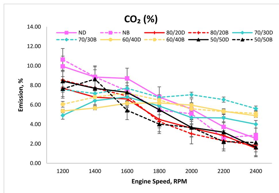
Figure 8. CO<sub>2</sub> emission at variable speed.
