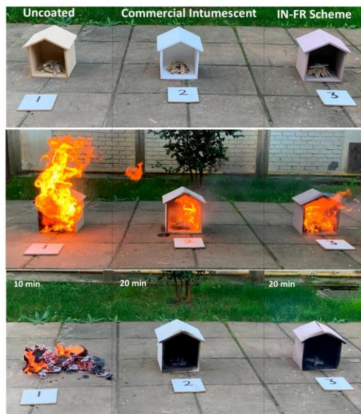
**Figure 5.** Field test of the dual scheme (IN-FR) on wood.
