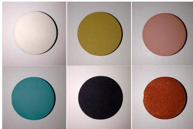
**Figure 5.** Colorful PEO coatings on the 6061 Al-alloy sample. Reprinted with permission from [110]; Copyright 2016 Elsevier. These colors have been created through in-situ incorporation of several organic dyes under constant voltage mode via path 5 in form of direct micro-emulsion.
