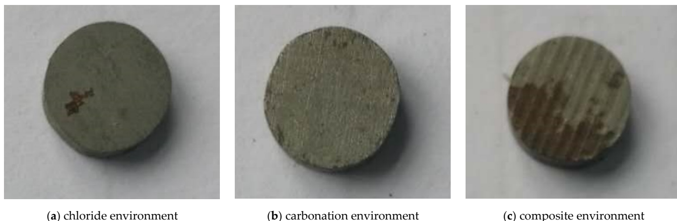
Figure 2. Corrosion state of steel wafers under different conditions.
