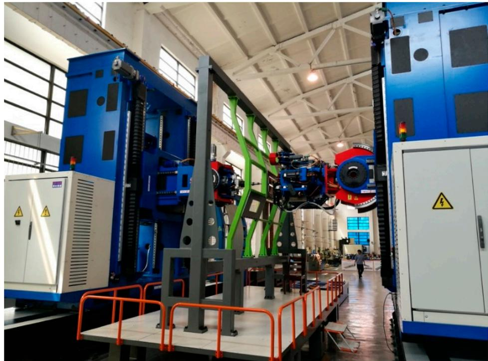
**Figure 8.** Automatic drilling and riveting machine pressure riveting test.
