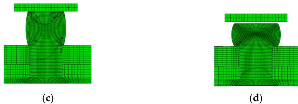
**Figure 1.** Riveting deformation process: (a) stage 1 of riveting process; (b) stage 2 of riveting process; (c) stage 3 of riveting process; (d) stage 4 of riveting process.
