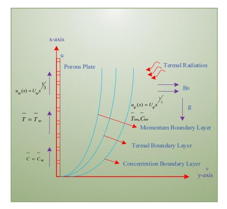
Figure 1. Flow geometry for HTM-BFN model with MHD.
