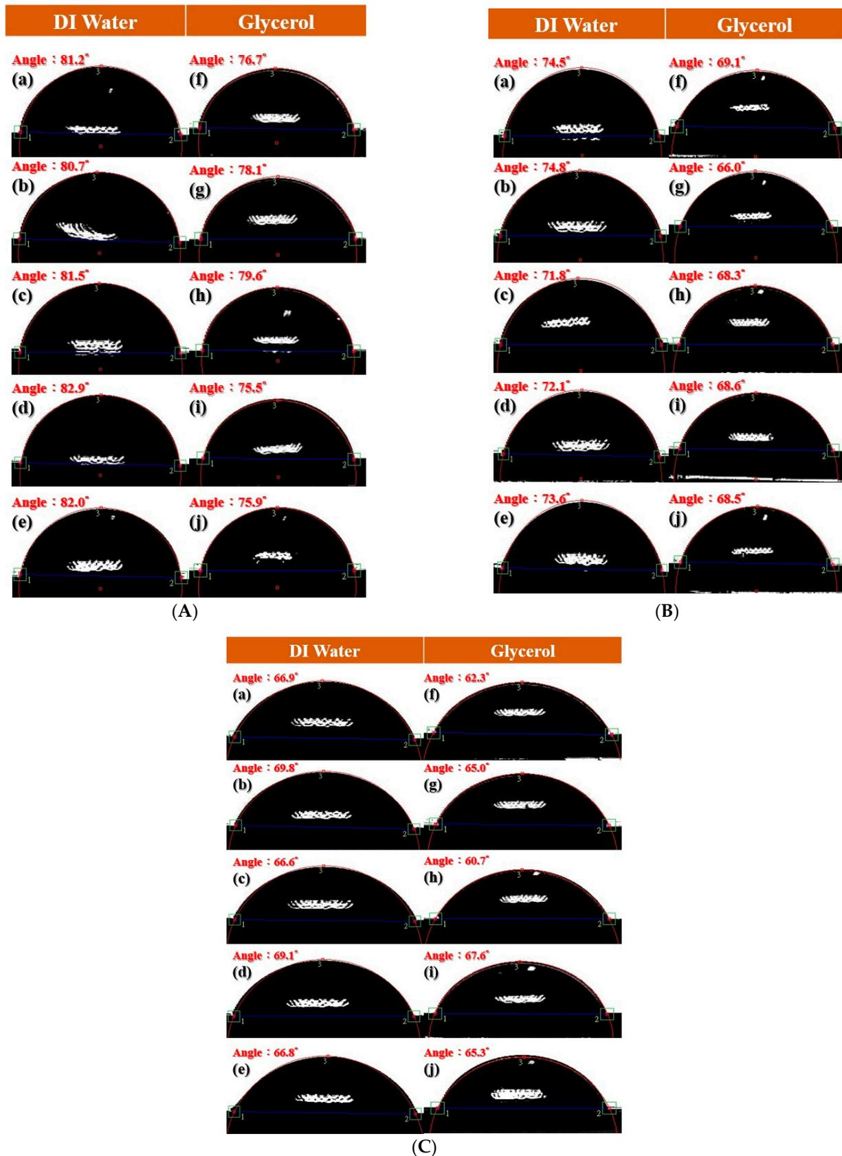
**Figure 3.** Contact angles of the  $\text{Co}_{40}\text{Fe}_{40}\text{W}_{20}$  thin films under three conditions: (A) as-deposited, (B) after post-annealing at  $250^\circ\text{C}$ , (C) after post-annealing at  $350^\circ\text{C}$  with DI water: (a) 10 nm, (b) 20 nm, (c) 30 nm, (d) 40 nm, and (e) 50 nm. Contact angles of the  $\text{Co}_{40}\text{Fe}_{40}\text{W}_{20}$  thin films with glycerol: (f) 10 nm, (g) 20 nm, (h) 30 nm, (i) 40 nm, and (j) 50 nm.
