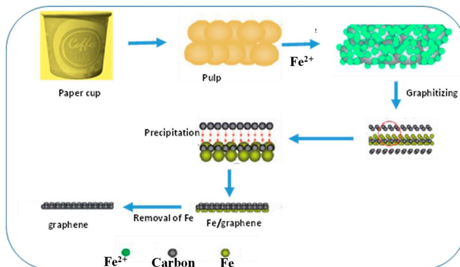
Figure 1. Formation mechanism of graphene sheets from paper cups [25].
