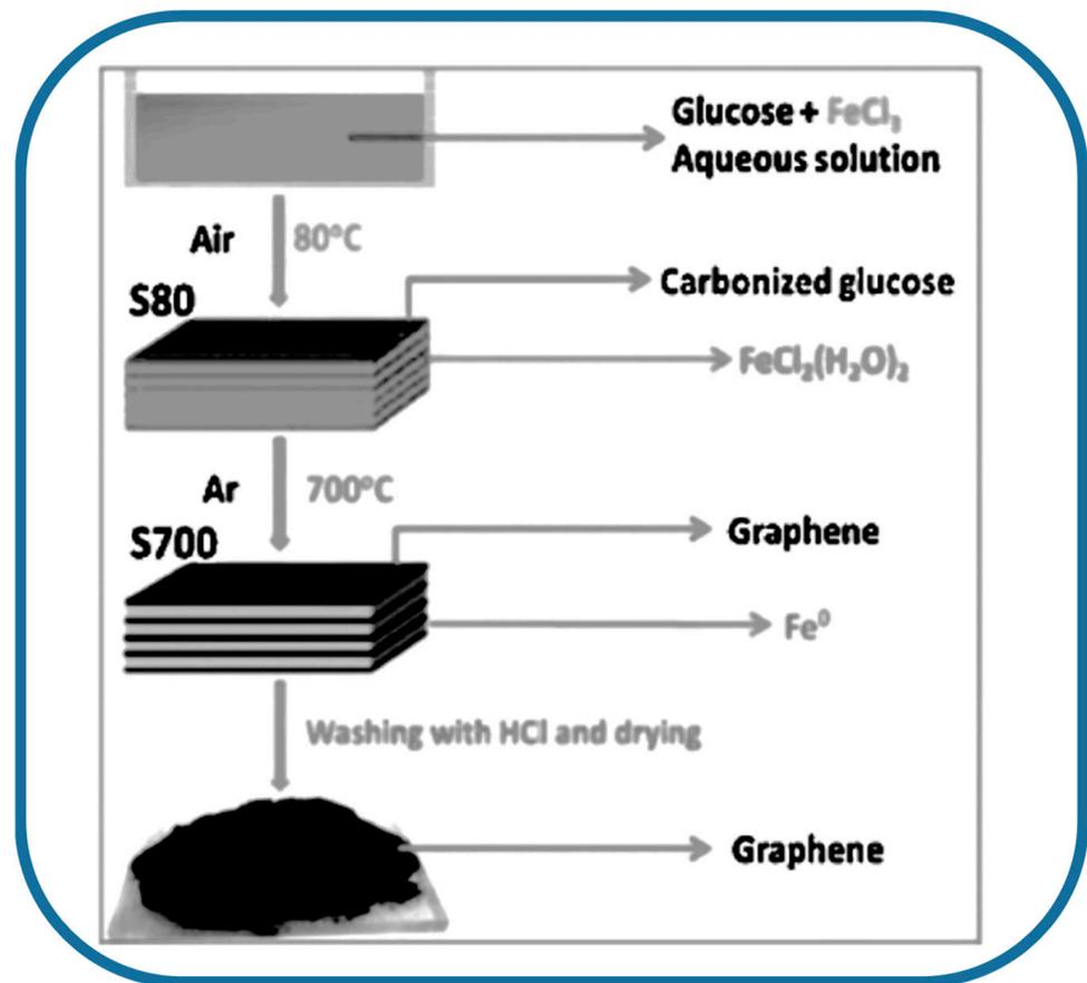
Figure 3. Preparation of graphene from glucose with the help of ferric chloride [37].
