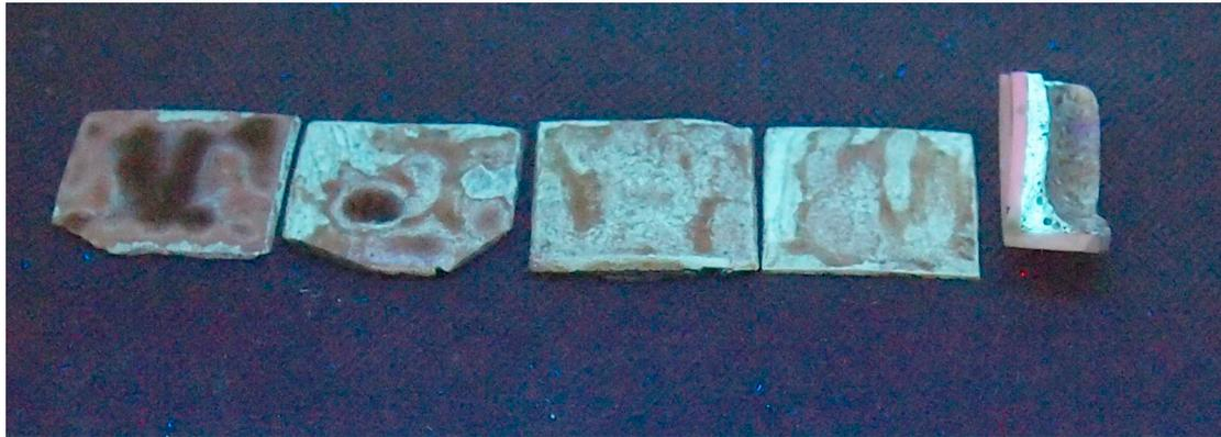
**Figure 8.** From the left: Coatings after CMAS interaction for 1, 4, 8 and 10 h and the cross-sectioned bottom of a crucible with sintered mixture of powders, respectively. Samples illuminated by the 312 nm lamp (i.e., 3.97 eV).
