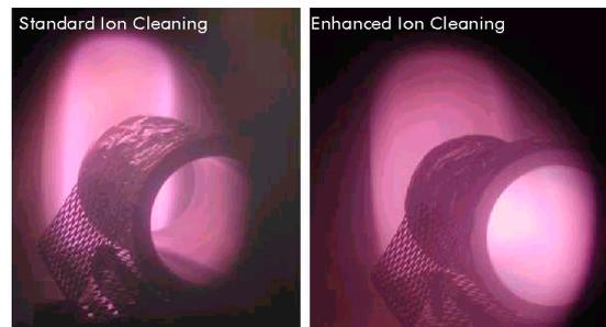
**Figure 3.** Photo shots (Gencoa, <https://www.gencoa.com/>) of cylinder liners in front of a Cr target during ion cleaning. The standard ion cleaning (**left**) does not allow plasma penetration, whilst the enhanced ion cleaning (**right**) allowed the desired penetration.
