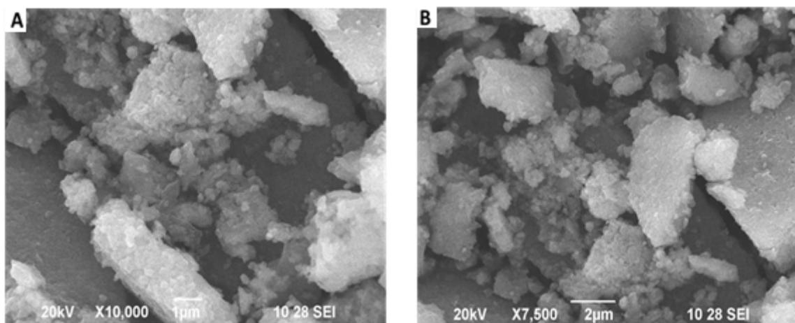
**Figure 2.** SEM images of selenium nanoparticles synthesized using *D. indica* plant broth. (A) 1  $\mu\text{m}$  view, (B) 2  $\mu\text{m}$  view.
