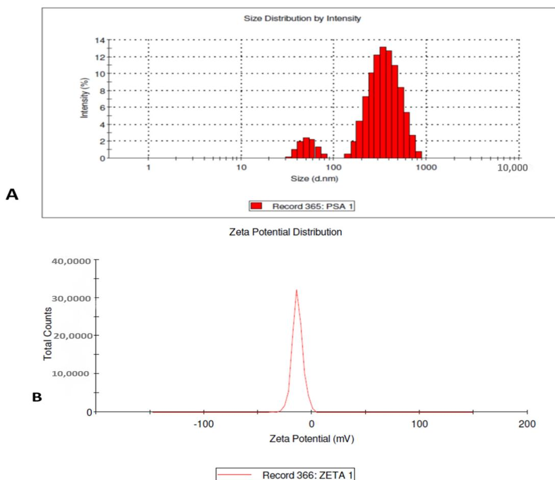
**Figure 3.** Dynamic light scattering (DLS) size distribution (A) and zeta potential analysis (B) of selenium nanoparticles synthesized using *D. indica*.
