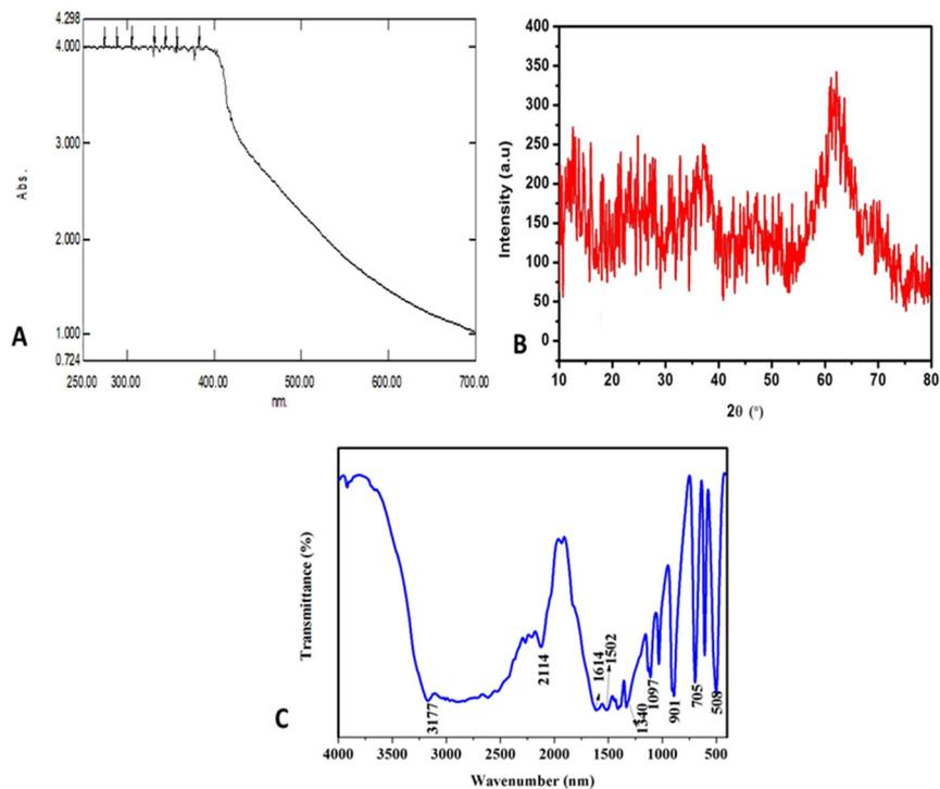
**Figure 1.** (A) Ultraviolet-visible spectra recorded, (B) XRD recorded and (C) FT-IR recorded of selenium nanoparticles synthesized using *D. indica* leaf broth.
