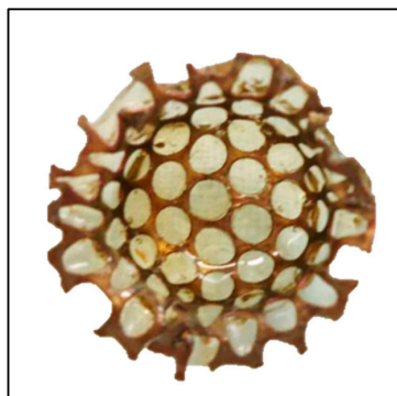
Figure 1. Titanium mesh dome shaped with a 10 mm diameter, coated with polymerized natural rubber latex.
