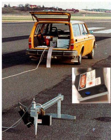
**Figure 1.** The VTI stationary profilometer, with its “macro” sensor mounted on the sled, and the “micro” sensor inserted in the photo, resized to approximately 5 times the scale of the rest of the photo. The photo was shot in another project.
