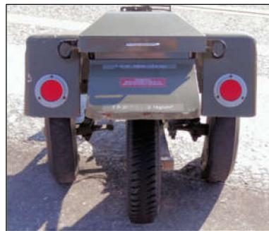
**Figure 3.** A Mu-meter with its two friction measuring tires at both sides of a free-rolling speed-measuring tire. The photo was shot in another project.
