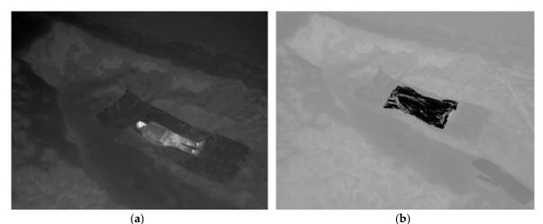
**Figure 2.** Thermal images in a snow-covered backcountry environment. (**a**) Model in supine position on an insulating sheet. (**b**) Model in supine position on an insulating sheet covered with a single-layer rescue blanket, silver side up. (**c**) Model in supine position on an insulating sheet covered with a single-layer rescue blanket, gold side up (air temperature: -6.2 °C; snow temperature: -7.6 or -6.3 °C when considering the emissivity coefficient  $\varepsilon = 0.83$  for snow).
