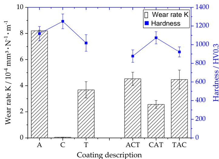
**Figure 7.** Hardness and sliding wear rates of plain oxide coatings (A, C, T) and composite coatings (ACT, CAT, TAC).
