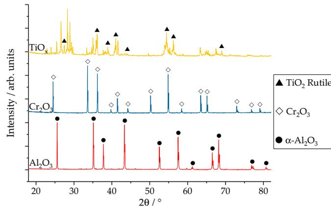
Figure 2. XRD pattern of the feedstock powders.
