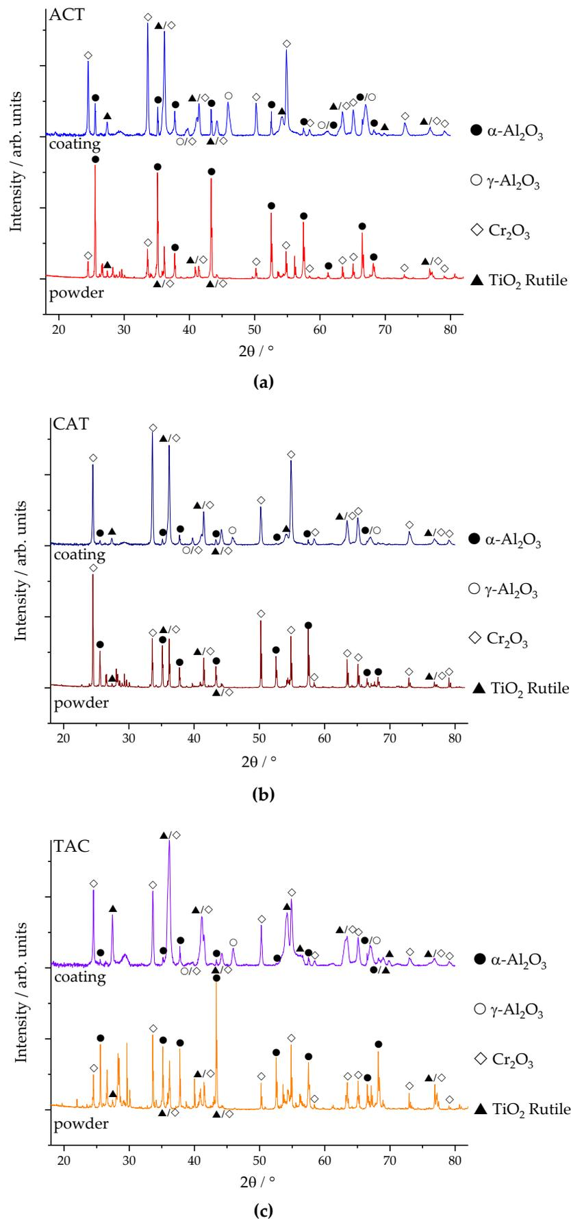
**Figure 8.** Diffraction patterns of the powder blends and corresponding coatings: (a) ACT, (b) CAT, and (c) TAC.
