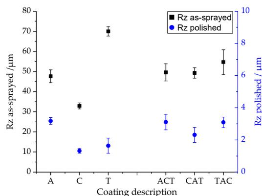
Figure 3. Roughness values of as-sprayed and polished coated samples.
