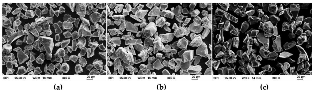
**Figure 1.** SEM images of the feedstock powders. (a)  $\text{Al}_2\text{O}_3$ . (b)  $\text{Cr}_2\text{O}_3$ . (c)  $\text{TiO}_x$ .
