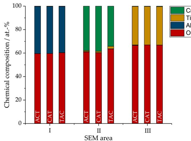
**Figure 6.** EDS analysis of composite coatings: chemical composition of the material areas marked in Figure 5b,d,f.
