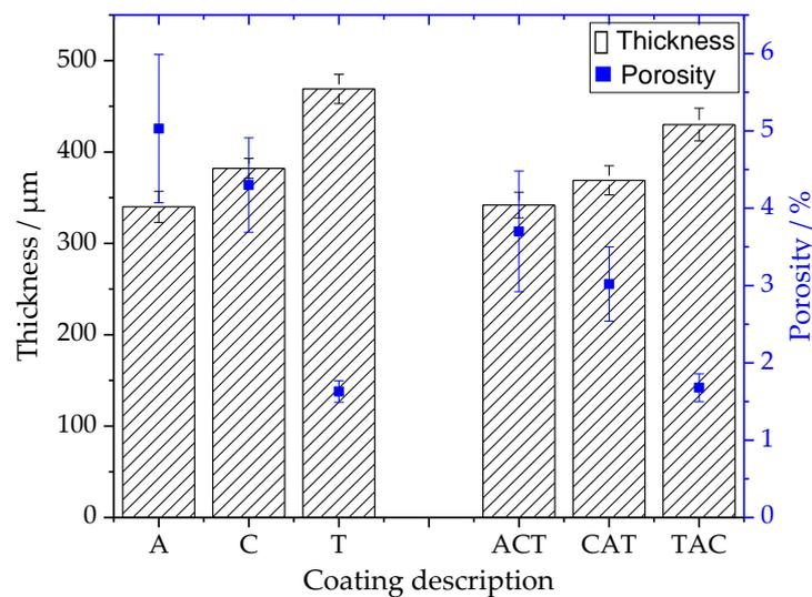
**Figure 4.** Thickness and porosity of plain oxide coatings (A, C, T) and coatings from blends (ACT, CAT, and TAC).
