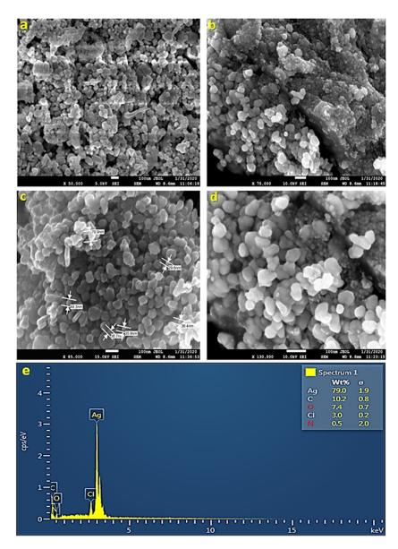
**Figure 5.** SEM-EDX spectra of biosynthesized silver nanoparticles. SEM images (**a**–**d**) of the AgNPs demonstrate that their spherical shape ranges from 29 to 70 nm in size. An elemental analysis of AgNPs was confirmed by EDX (**e**), which reveals that 79% of the material is made up of Ag. A strong peak signal was observed at 3 KeV, which is characteristic of metallic AgNPs absorption.
