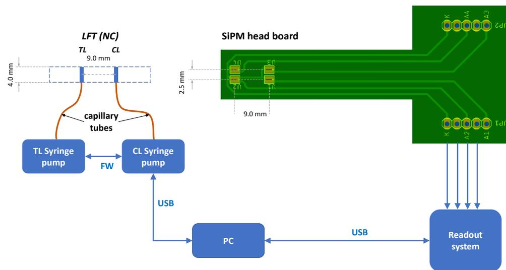
**Figure 2.** Layout of the connections of the biosensor, showing the main block components. **(Left)** developer delivery subsystem, **(Right)** the SiPM head board connections.
