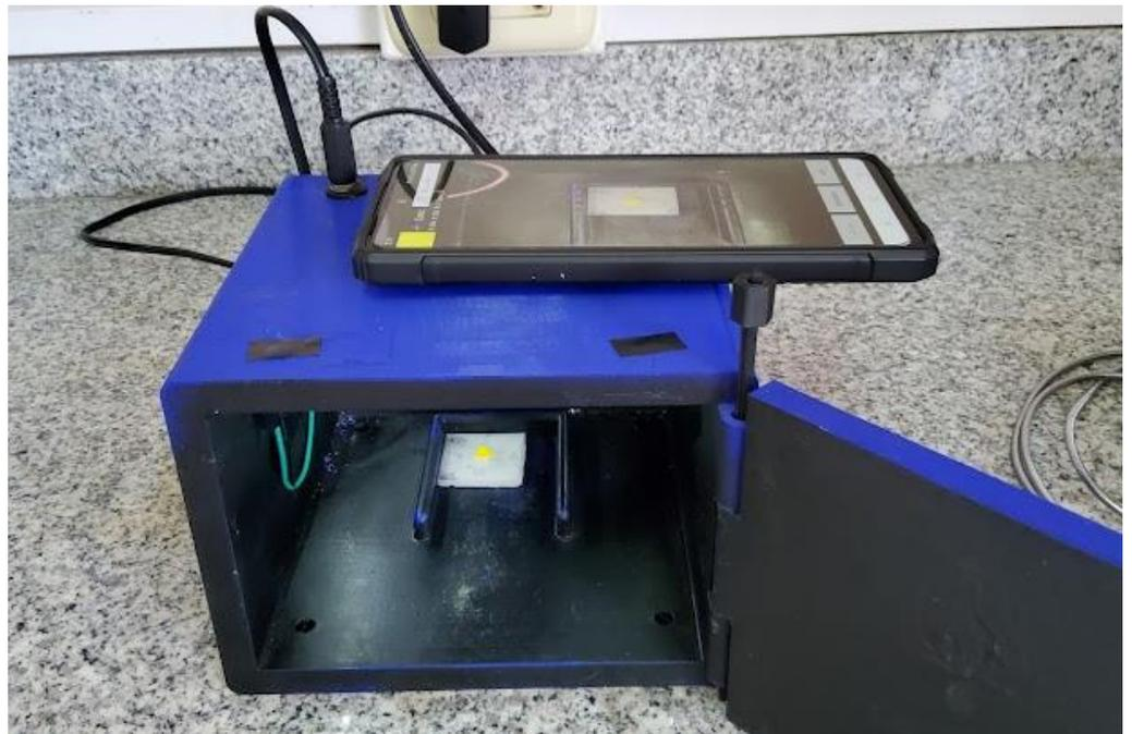
**Figure 2.** RadesPhone device with the smartphone for imaging the MIP on the sample holder.
