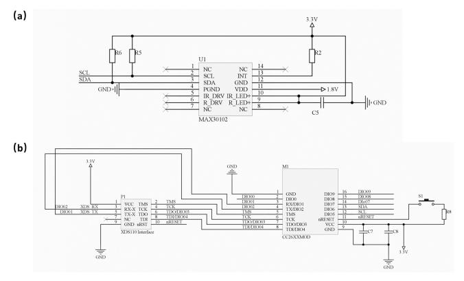
Figure 2. The photoelectric sensor module circuit (a); The BLE and MCU module circuit (b).
