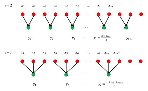
Figure 9. Coarse grain sequences for scale 2 and 3.
