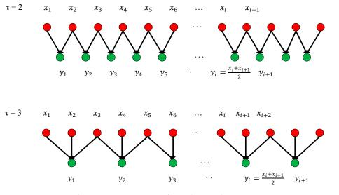
Figure 10. Improved time series coarsening for scales 2 and 3.
