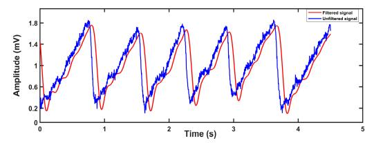
Figure 14. Filtered effect of digital IIR filter.
