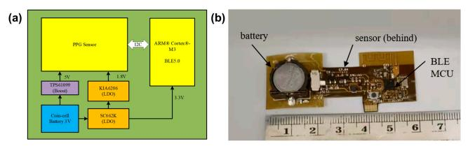
**Figure 1.** Circuit architecture of the smart ring for the apnea diagnosis (**a**), Photo of the fabricated FPC circuit board (**b**).
