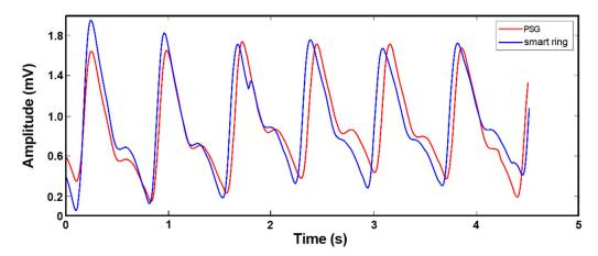
**Figure 13.** Pulse waves collected by the smart ring (blue) and a professional polysomnograph instrument (red), respectively.
