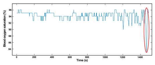
**Figure 7.**  $SpO_2$  level variation with time for a wearer is measured by our smart ring. The significantly low  $SpO_2$  level at the time of 1480 s indicates the sleeping apnea of the wearer.
