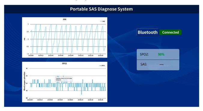
**Figure 5.** App graphics user interface developed to receive the PPG signal from the smart ring during sleep.
