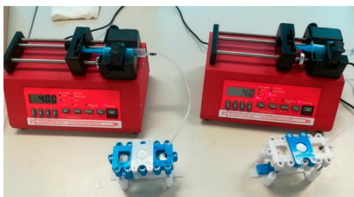
Figure 13. The experimental setup consists of two simultaneous skins-on-a-chip [119]. This setup contains a flow-through dynamic microfluidic device and a programmable syringe pump. The experimental samples can be collected below the diffusion system in the collection bench. Reproduced with permission from MDPI Copyright (2023).
