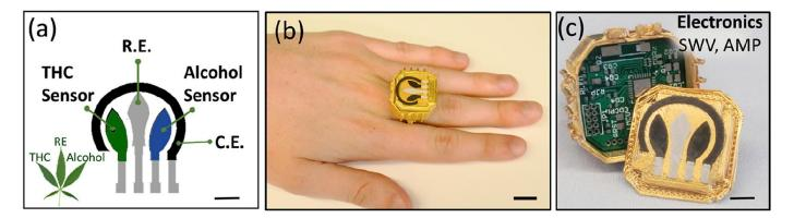
**Figure 4.** (a): The leaf-like sensor configuration, including dual working electrodes with the same counter electrode (C.E.) and reference electrode (R.E.). (b): Wearable electrochemical ring sensor. (c): The case, electronic board, and sensing system. Reprinted and adapted from ref. [45]. Copyright 2020 Elsevier.
