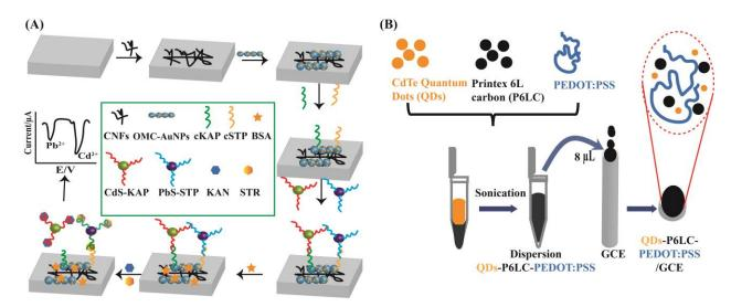
**Figure 5.** Nanomaterial-based electrochemical methods for antibiotic analysis. (**A**) The ultrasensitive electrochemical detection of kanamycin and streptomycin carbon nanofibers and mesoporous carbongold nanoparticles [40]. (**B**) An electrochemical device for the determination of amoxicillin based on a combination of nanomaterials such as Printex 6 L Carbon and cadmium telluride quantum dots within a poly(3,4-ethylenedioxythiophene) polystyrene sulfonate film [41].
