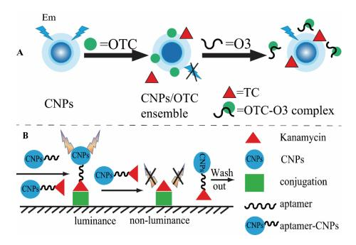
**Figure 6.** Carbon nanoparticle-based fluorescence methods for the determination of antibiotics. **(A)** Competitive analysis for oxytetracycline, based on aptamer and carbon nanoparticles [48].
