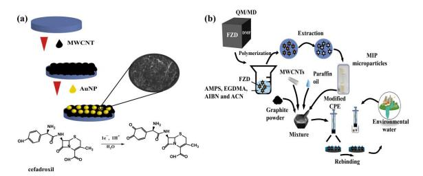
**Figure 3.** (a) The determination of cefadroxil β-lactam antibiotic was carried out using a modified gold nanoparticle/multiwalled glassy carbon nanotube [34]. (b) Molecularly imprinted carbon paste electrode for furazolidone detection [35].
