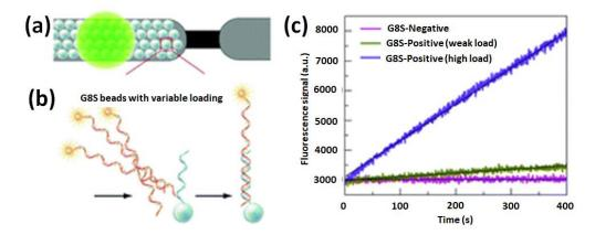
**Figure 14.** (a) Schematic microfluidic microarray hybridization on tightly packed monolayer bead bed inside a microfluidic cartridge for the detection of single-nucleotide polymorphisms; (b) real-time monitoring of DNA hybridization on spherical particles functionalized with oligonucleotide capture probes nominated as G8S. (c) Fluorescence emission detection from real-time monitoring of DNA hybridization events vs. the pass of time. Reprinted with permission ref. [118]. Copyright 2021, RSC.
