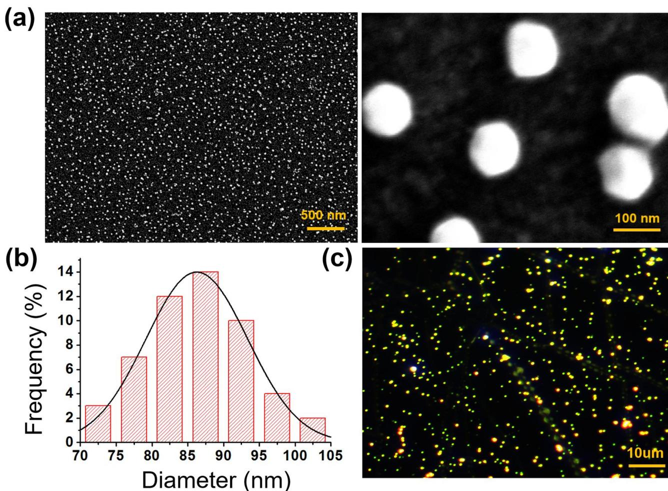
**Figure 2.** (a) SEM images, (b) frequency distribution curve, and (c) DFM of the flexible biosensor constructed using 80 nm AuNPs.
