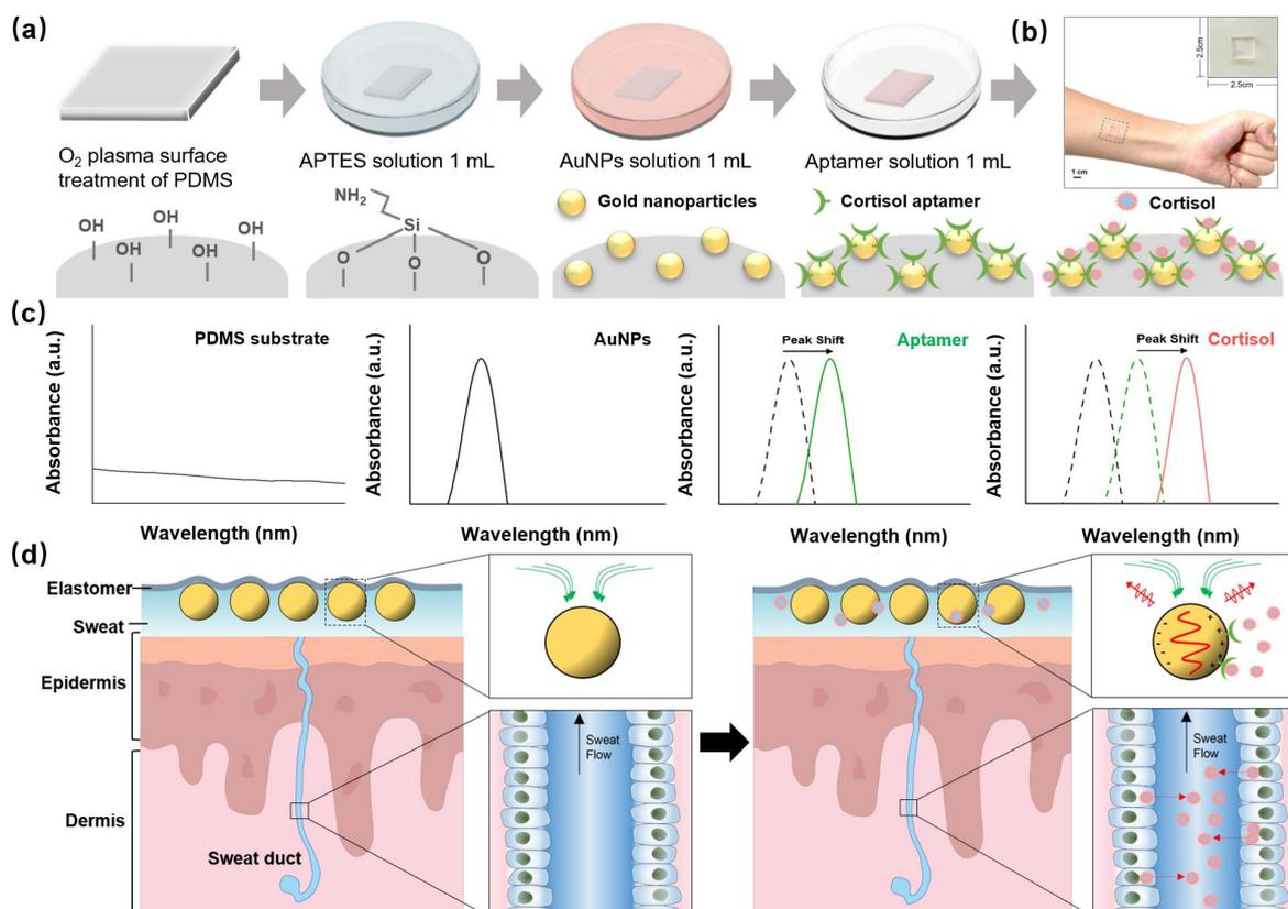
**Figure 1.** Schematic of the wearable sweat biosensor. (a) Fabrication process, (b) optical photography (c) reaction mechanism, and (d) structure of the human sweat gland showing the flexible LSPR biosensor interaction in the skin cross-section.
