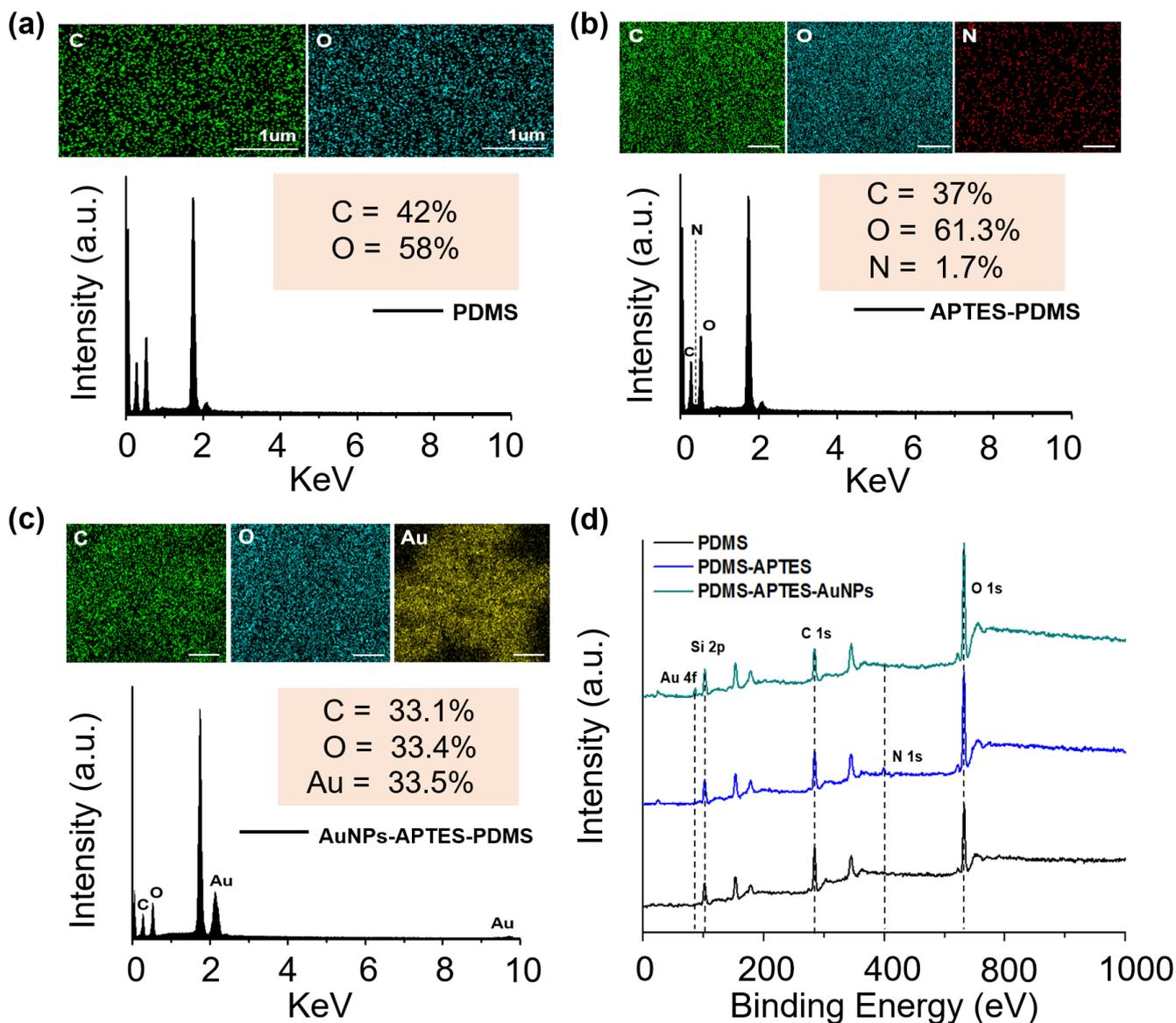
**Figure 3.** Characterization of the fabricated samples. EDX elemental analysis of (a) PDMS substrate, (b) PDMS-APTES, and (c) PDMS-APTES-AuNPs. (d) XPS curves of the LSPR biosensor.
