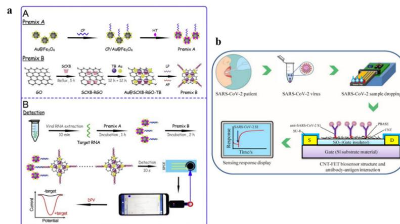
**Figure 3.** Schematic illustration of electrochemical biosensors fabricated with carbon nanomaterials for detection of SARS-CoV-2: (a) biosensor based on graphene oxide with calixarene functionality for detecting RNA of SARS-CoV-2 via a smartphone [64]; (b) biosensor based on CNT-FET for detecting SARS-CoV-2 S1 antigens [79]. Note: (a,b) are reproduced with permission Copyright 2021, Elsevier B.V.
