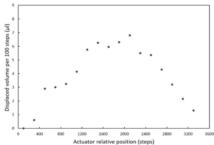
Figure A3. Dependence of the volume displaced by the pumping chamber on the relative position of the actuator.
