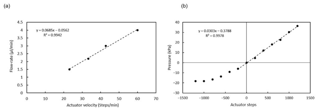
**Figure 5.** (a) Calibration of the flow rate vs. actuator velocity; (b) Calibration of the pressure vs. actuator displacement (all valves closed). Dashed lines are guides to the eye.
