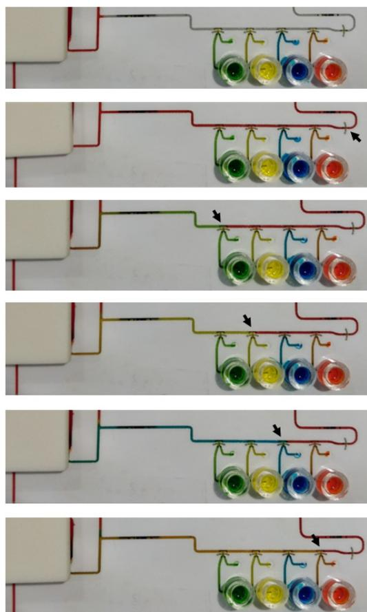
**Figure A4.** Images of the chip at different steps of an assay-like test. The black arrows indicate the open valves.
