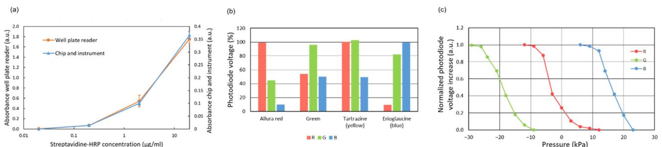
**Figure 6.** (a) Absorbance measurement for oxidized TMB. Comparative with a plate reader; (b) Photodiode output voltage signal for different dye solutions (and different activated LEDs) in relation to the values obtained for deionized water. The concentration of dyes is the same used for the reagents; (c) Calibration of the pressure measurement based on the compression of air in a dead-end channel.
