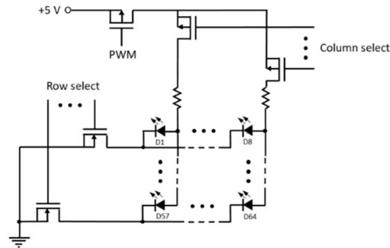
Figure A1. Circuit for LED row-column addressing.
