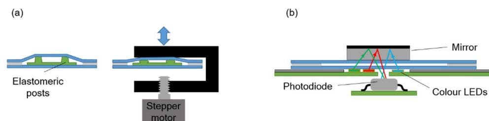
**Figure 2.** Schematic illustration of (a) the pumping system, and (b) the absorbance measurement system.
