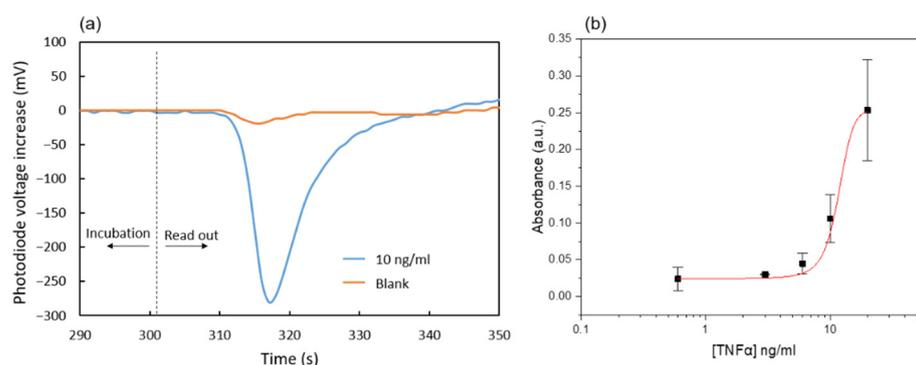
**Figure 7.** (a) Photodiode signals for two TNF $\alpha$  concentrations; (b) Absorbance response to different TNF $\alpha$  concentrations. Each data point is the average of three measurements obtained from three separate chips. The mean absorbance value of the blanks has been subtracted from the absorbance values obtained for all other TNF $\alpha$  concentrations.
