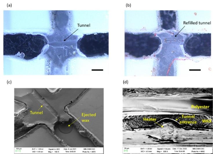
Figure A2. Microscope images of valves with the bottom polyester layer removed (a) after opening, and (b) after closing. Scale bars are 250  $\mu\text{m}$ ; (c) SEM image of an open valve with the bottom polyester layer removed; (d) SEM image of an open valve from the tunnel entrance side.
