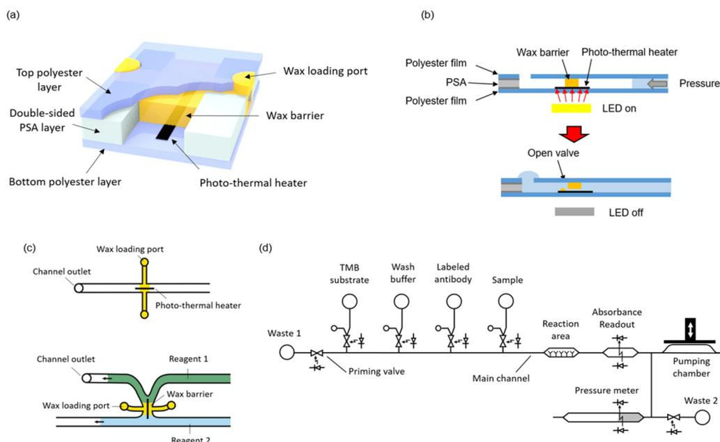
**Figure 1.** (a) A 3D illustration of the valve structure; (b) Cross-sectional representation of the valve opening; (c) Two different configurations of the wax valve; (d) Complete fluidic schematic of the ELISA chip.
