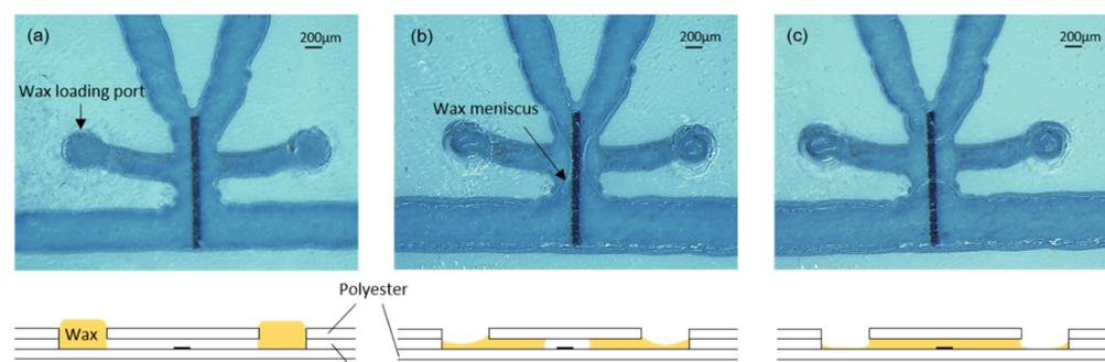
**Figure 3.** (a) Valve with wax-loading port full of wax; (b) Penetration of the wax inside the channel by capillarity; (c) Formation of the wax barrier on top of the heater. Bottom drawings are cross-sectional illustrations of the process.
