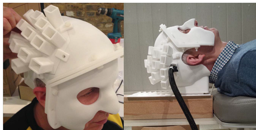
Figure 19. The 3D printed head model used for the experiments [130].
