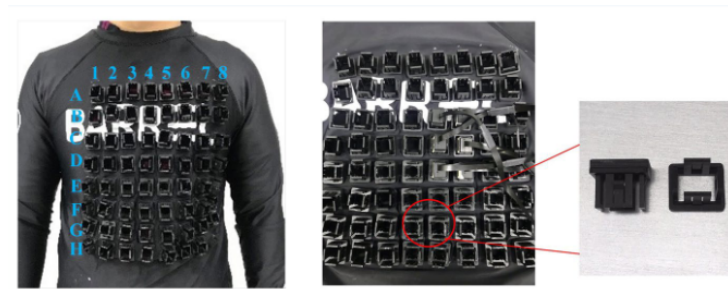
Figure 15. Position labels of the 8 \times 8 array with 30 mm intervals, QZFM magnetometer and customized receptacles [127].
