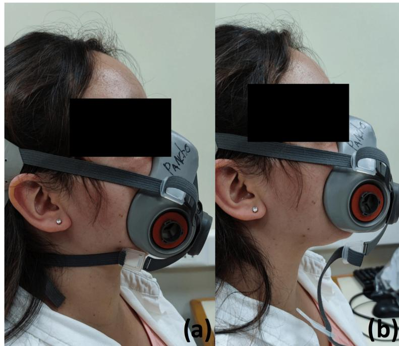
**Figure 7.** Volunteer with the reusable respirator in fitted (a) and loose (b) position.
