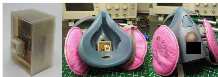
**Figure 4.** Implemented breathing monitoring embedded electronic device (left) inside a reusable respirator (center), where the positioning of the system is through an externally located magnet (right). The first image shows the embedded electronic device with epoxy resin.
