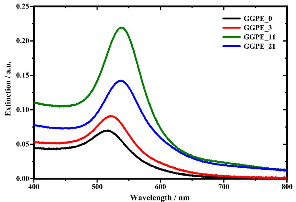
Figure 2. Localized surface plasmon band (LSPR) of the GGPE<sub>0</sub>, GGPE<sub>3</sub>, GGPE<sub>11</sub>, and GGPE<sub>21</sub> sample.
