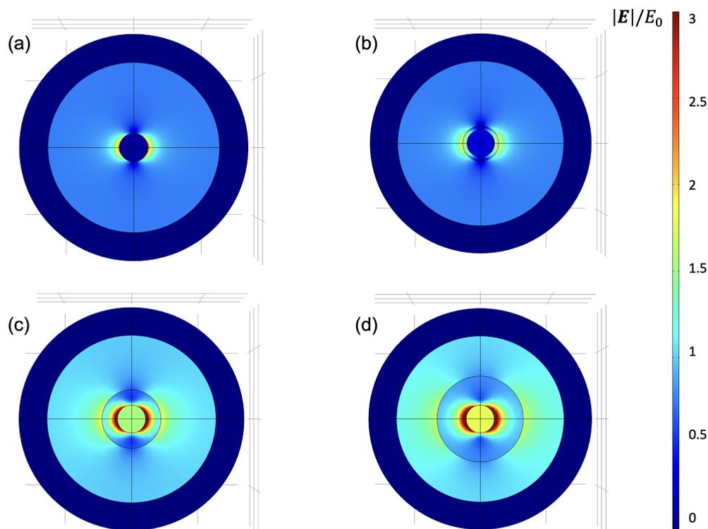
**Figure 7.** Finite element method (FEM) simulations reporting the local enhancement near-field around (a) GGPE<sub>0</sub>, (b) GGPE<sub>3</sub>, (c) GGPE<sub>11</sub>, and (d) GGPE<sub>21</sub>.
