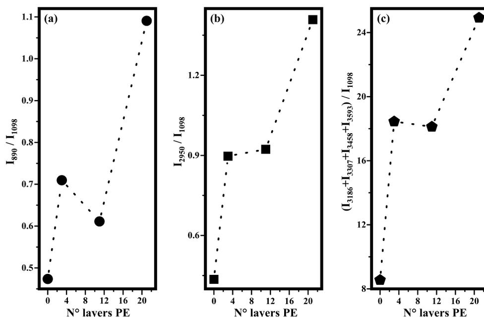
**Figure 6.** Trends, as a function of the number of the PE layers, of the ratios of intensities bands that fall at frequencies indicated as subscripts in  $I_{890}/I_{1098}$  (a),  $I_{2950}/I_{1098}$  (b), and  $(I_{3186} + I_{3307} + I_{3458} + I_{3593})/I_{1098}$  (c) and that have been calculated by the fitting procedure shown above (see Figure 4).
