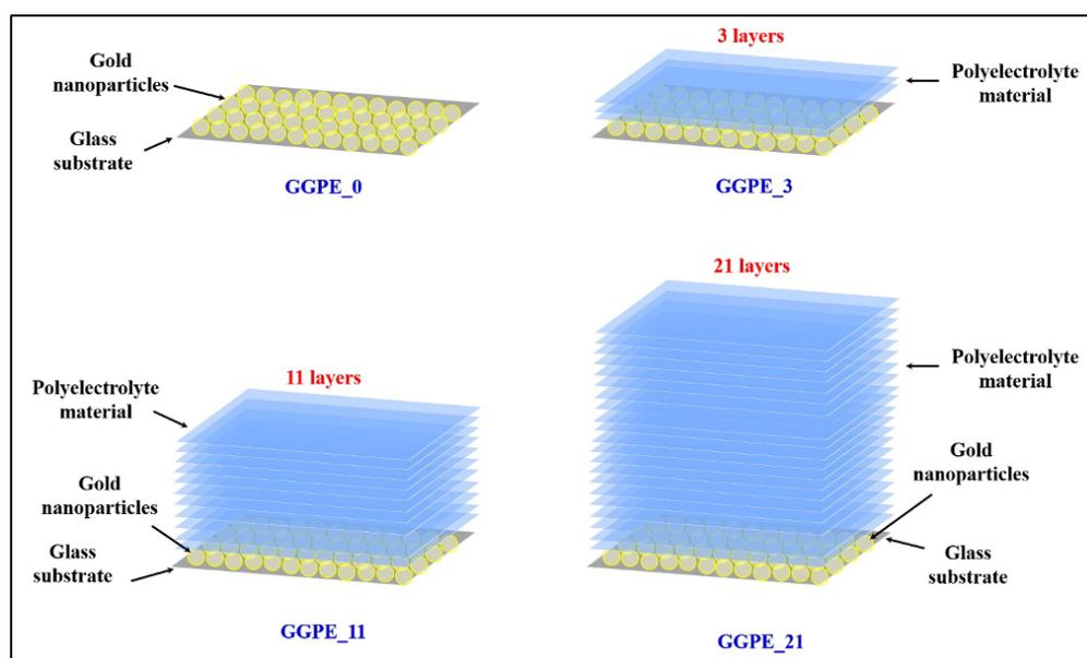
**Figure 1.** Schematic view of the four samples: GGPE<sub>0</sub> (glass substrate/GNPs), GGPE<sub>3</sub> (glass substrate/GNPs/3 layers of PE material), GGPE<sub>11</sub> (glass substrate/GNPs/11 layers of PE material), and GGPE<sub>21</sub> (glass substrate/GNPs/21 layer of PE material).
