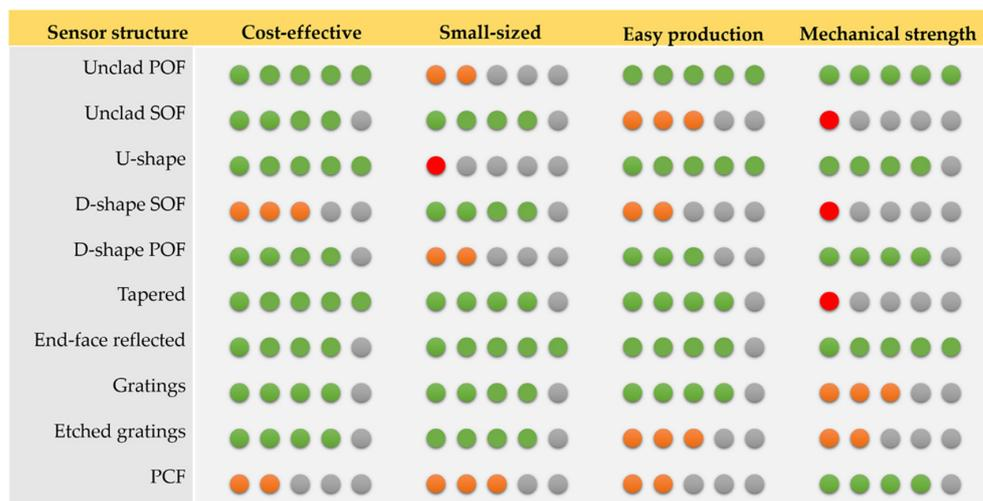
**Figure 5.** Infographic of the main characteristics of several optical fiber structures (green: great–good; orange: medium–fair; red: poor).
