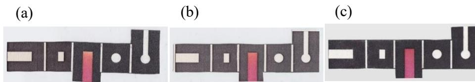
**Figure S4.** Image of sensor with a) 20.0  $\mu\text{L}$  b) 30.0  $\mu\text{L}$  and c) 50.0  $\mu\text{L}$  of murexide solution
