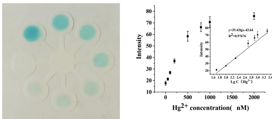
**Figure 5.** The image of detection of  $\text{Hg}^{2+}$  and calibration curve of colorimetric detection.
