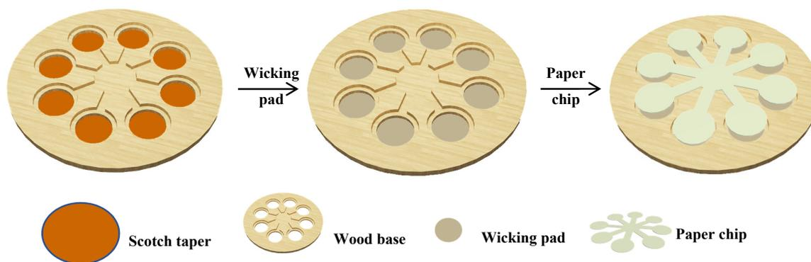
Figure 1. Schematic of paper device fabrication.
