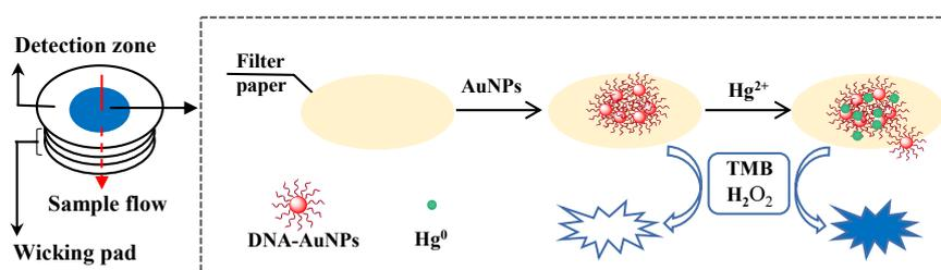
Figure 2. Schematic diagram of  $\text{Hg}^{2+}$  detection.
