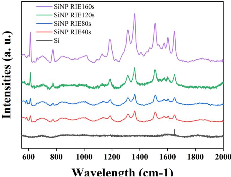
Figure S2. Raman spectra of R6G on nanopillars (RIE 40–160 s) and bare silicon.
