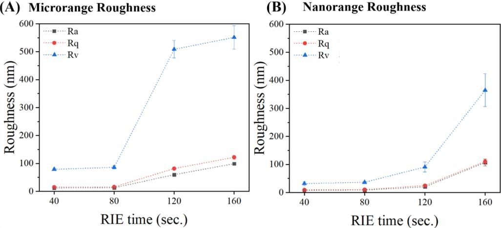
Figure S1. (A) AFM analysis data for (A) microrange and (B) nanorange roughness. Roughness is presented as Ra (black), Rq (red), and Rv (blue) in our AFM software.
