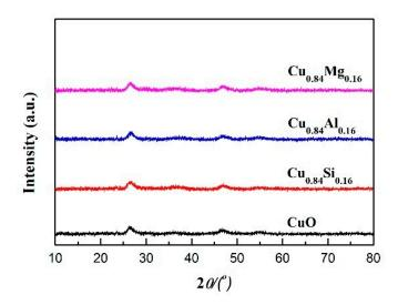
Figure 8. XRD patterns of used catalysts.
