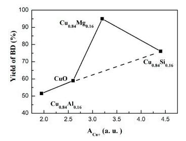
**Figure 13.** The BD yield of catalysts after 15 h as a function of the integrated area of the Cu<sup>+</sup> peak  $(A_{Cu+})$  determined by CO-IR spectroscopy.
