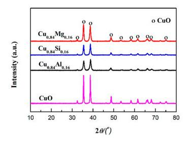
Figure 1. X-ray diffraction (XRD) patterns of the catalysts.
