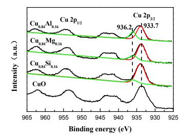
Figure 3. Cu 2p X-ray photoelectron spectroscopy (XPS) spectra of the catalysts.
