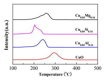
Figure 4. H<sub>2</sub>- temperature-programmed reduction (TPR) profiles of the catalysts.
