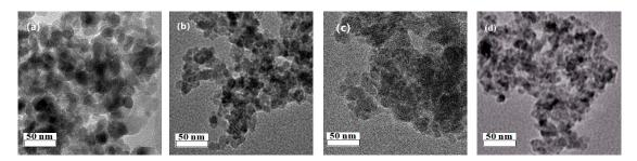
Figure 2. TEM images of (a) CuO, (b) Cu<sub>0.84</sub> Si<sub>0.16</sub>, (c) Cu<sub>0.84</sub>Mg<sub>0.16</sub>, and (d) Cu<sub>0.84</sub>Al<sub>0.16</sub>.
