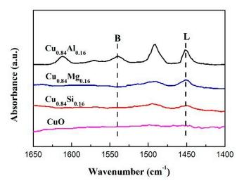
Figure 7. In situ Py-IR spectra of the catalysts.
