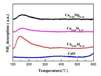
Figure 6. NH<sub>3</sub>-TPD profiles of the catalysts.
