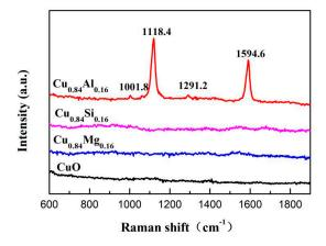
Figure 10. Raman spectra of used catalysts.
