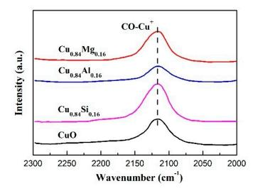
Figure 9. CO-IR spectra of used catalysts.
