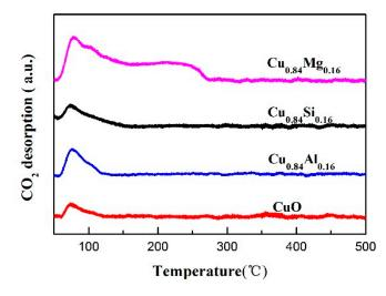
Figure 5. CO<sub>2</sub>- temperature-programmed desorption (TPD) profiles of the catalysts.
