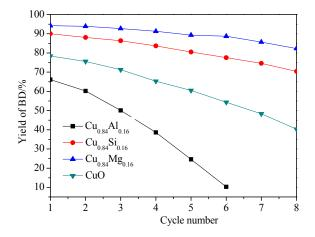
**Figure 12.** The yield of BD by CuO and Cu<sub>0.84</sub> $M_{0.16}$  catalysts as a function of the cycle number. Reaction conditions: Catalyst amount, 2.5 g; formaldehyde solution concentration, 35 vol.%; consumption of the formaldehyde solution, 50 mL; reaction temperature, 90°C, reaction time, 24 h.
