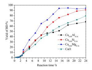
**Figure 11.** The yield of 1,4-butynediol (BD) by CuO and  $Cu_{0.84}M_{0.16}$  catalysts. Reaction conditions: Catalyst amount, 2.5 g; formaldehyde solution concentration, 35 vol.%; consumption of the formaldehyde solution, 50 mL; reaction temperature, 90°C.
