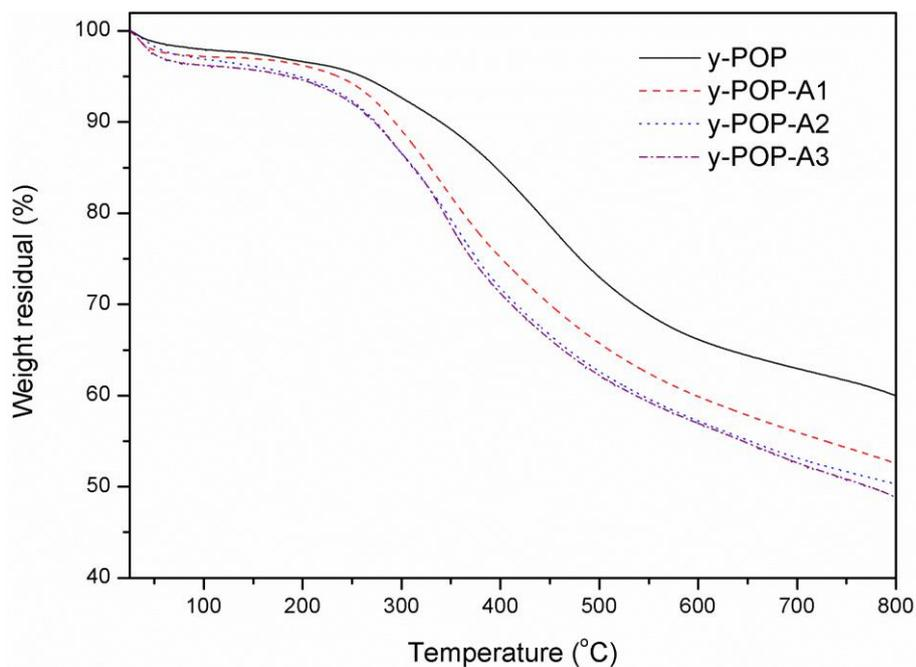
**Figure S1.** Thermogravimetric analysis curves of y-POP and y-POP-NH<sub>2</sub>.
