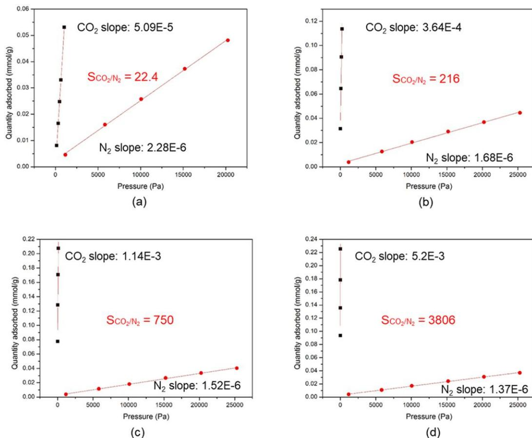
**Figure S9.** The CO<sub>2</sub> and N<sub>2</sub> adsorption data of (a) y-POP, (b) y-POP-A1, (c) y-POP-A2, and (d) y-POP-A3 at low partial pressures at 273 K and the linearly fitted results. Henry's law CO<sub>2</sub>-over-N<sub>2</sub> selectivities were calculated from the initial slopes of the CO<sub>2</sub> and N<sub>2</sub> isotherms.
