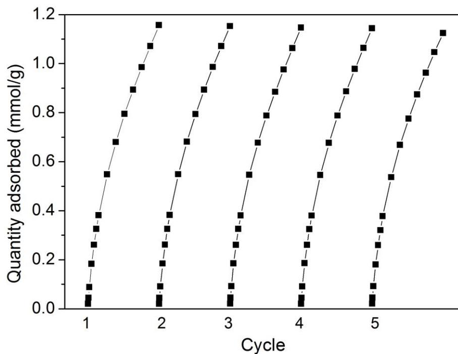
**Figure S6.** CO<sub>2</sub> adsorption-desorption cycles for y-POP-A1 recorded at 293 K.
