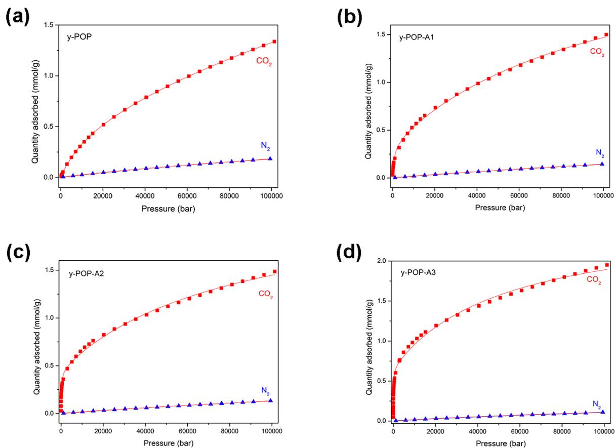
**Figure S8.** CO<sub>2</sub> (■) and N<sub>2</sub> (▲) adsorption data and of y-POP and y-POP-NH<sub>2</sub> recorded at 273 K. The red solid lines show the fitting results of the data: The CO<sub>2</sub> and N<sub>2</sub> adsorption data was fitted by a dual-site and single-site Langmuir model, respectively. Detail fitting results are given in Table S1. The fitted parameters from the single adsorption data were used to predict the IAST selectivity.
