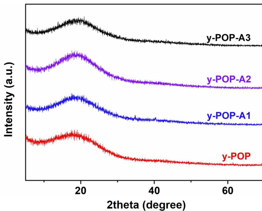
**Figure S4.** Powder X-ray diffraction patterns of y-POP and y-POP-NH<sub>2</sub> showing the polymers are mainly amorphous.
