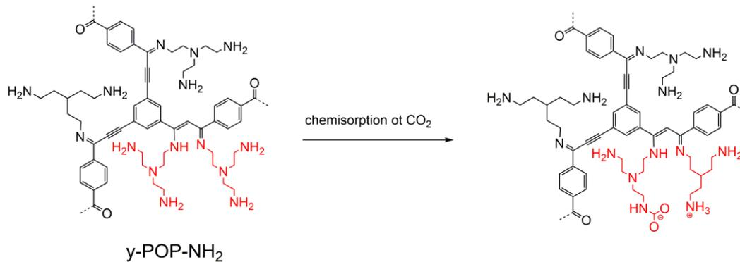
**Scheme S1.** Possible mechanism of chemisorption of CO<sub>2</sub> on y-POP-NH<sub>2</sub> with high amine loadings.
