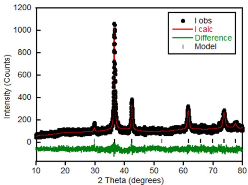
**Figure S6:** Refinement profile for the Rietveld analysis of room temperature XRD data that was collected for 6.0 V and fitted to the model.<sup>S1</sup>
