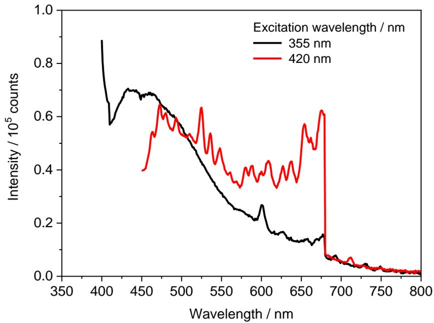
**Figure S13:** Emission spectra for commercial Cu<sub>2</sub>O.
