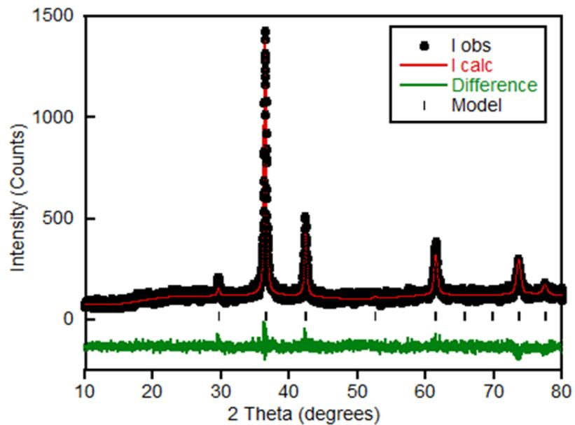
**Figure S5:** Refinement profile for the Rietveld analysis of room temperature XRD data that was collected for 5.0 V and fitted to the model.<sup>S1</sup>
