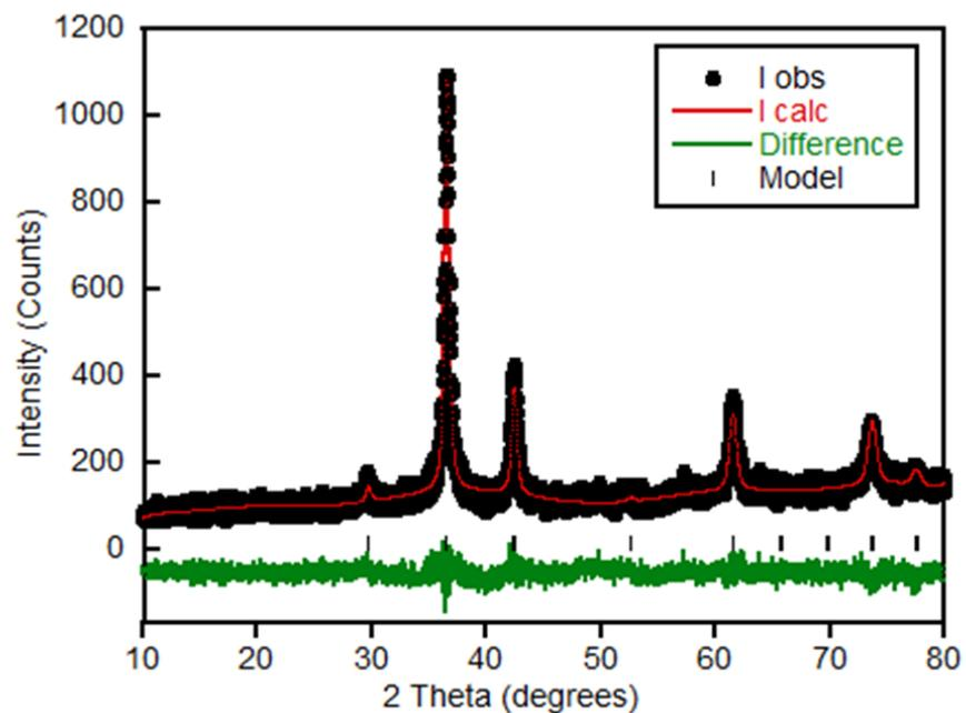
**Figure S7:** Refinement profile for the Rietveld analysis of room temperature XRD data that was collected for 7.0 V and fitted to the model.<sup>S1</sup>
