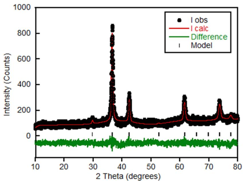
**Figure S8:** Refinement profile for the Rietveld analysis of room temperature XRD data that was collected for 8.0 V and fitted to the model.<sup>S1</sup>
