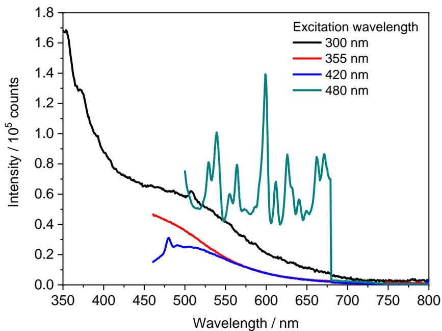
**Figure S10:** Emission spectra for Cu<sub>2</sub>O synthesized by bipolar electrochemistry at 4.5 V (3h).
