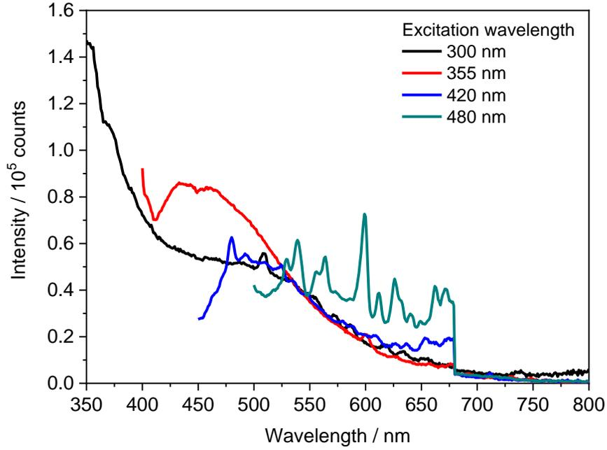
**Figure S12:** Emission spectra for Cu<sub>2</sub>O synthesized by bipolar electrochemistry at 8.0 V (1h).
