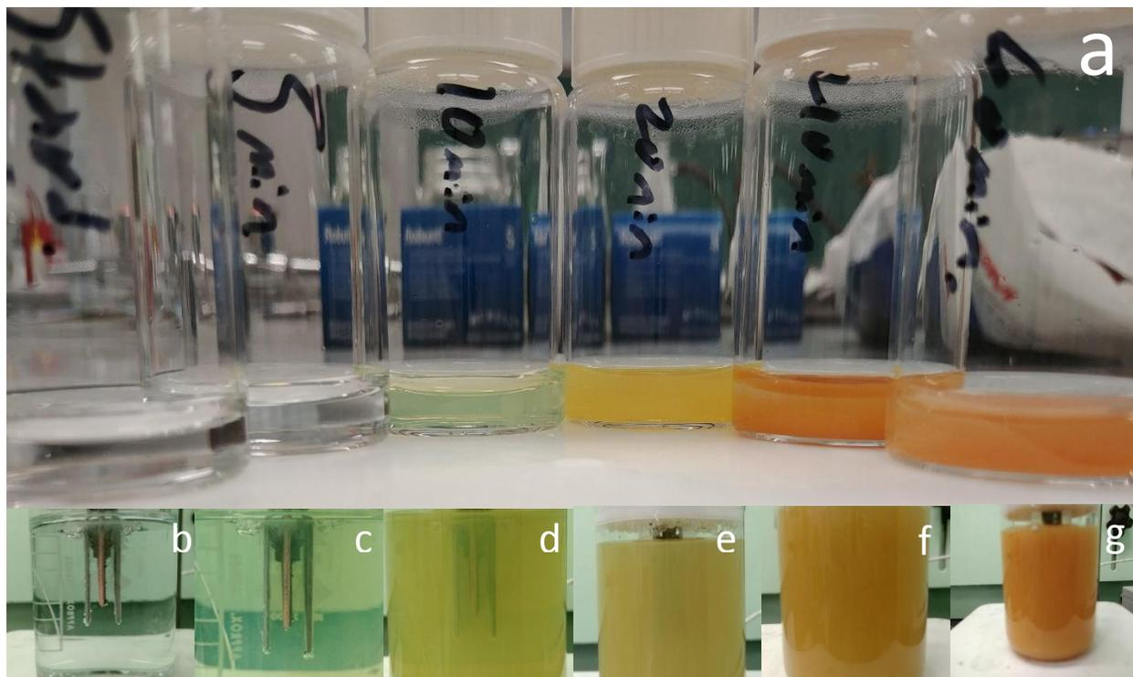
**Figure S2:** (a) Color change of the reaction solution during BPE synthesis over 60 min, from left: 0 min, 10, 20, 30, 40 and 60 min (right photo). (b-g) Photos taken during progression of the reaction inside the bipolar cell.
