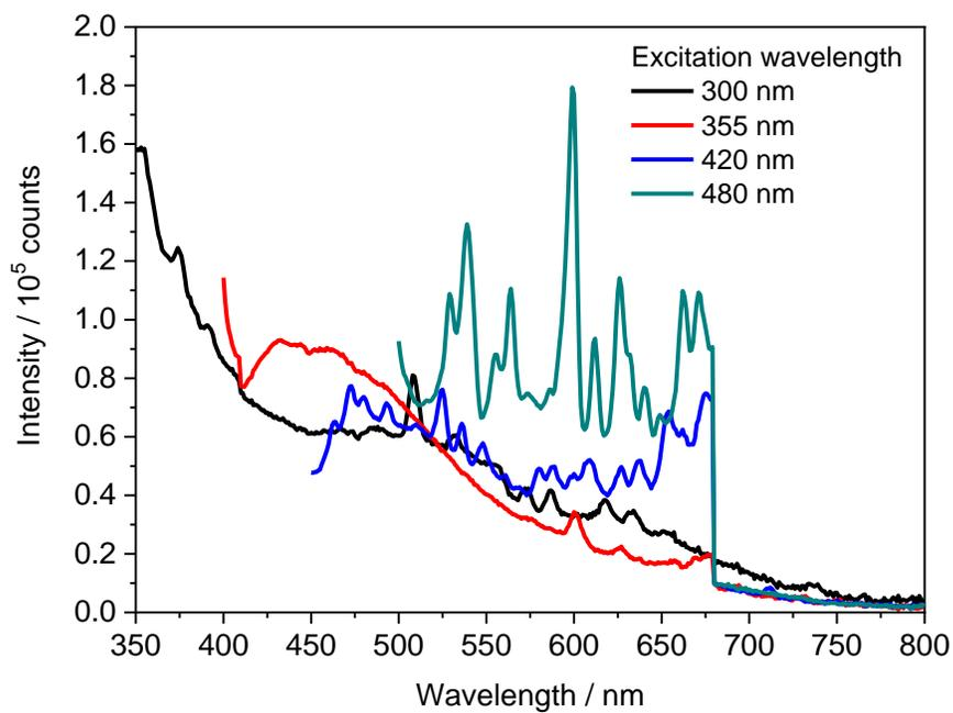
**Figure S11:** Emission spectra for Cu<sub>2</sub>O synthesized by bipolar electrochemistry at 6.0 V (1h).
