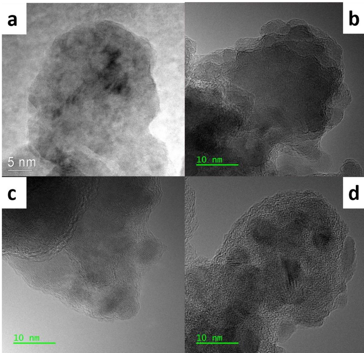
**Figure S14:** TEM of  $\text{Cu}_2\text{O}$  synthesized by bipolar electrochemistry for 1 hour at 4.5 V (a), 6.0 V (b), 7.0 V (c) and 8.0 V (d).
