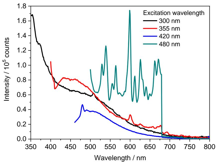
**Figure S9:** Emission spectra for Cu<sub>2</sub>O synthesized by bipolar electrochemistry at 4.5 V (1h).
