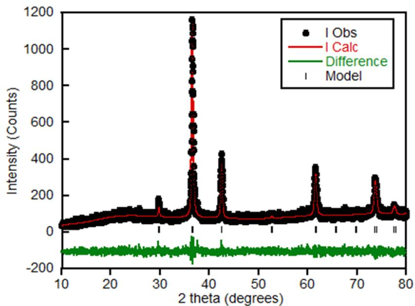
**Figure S3:** Refinement profile for the Rietveld analysis of room temperature XRD data that was collected for 4.5 V-3H and fitted to the model.<sup>S1</sup>
