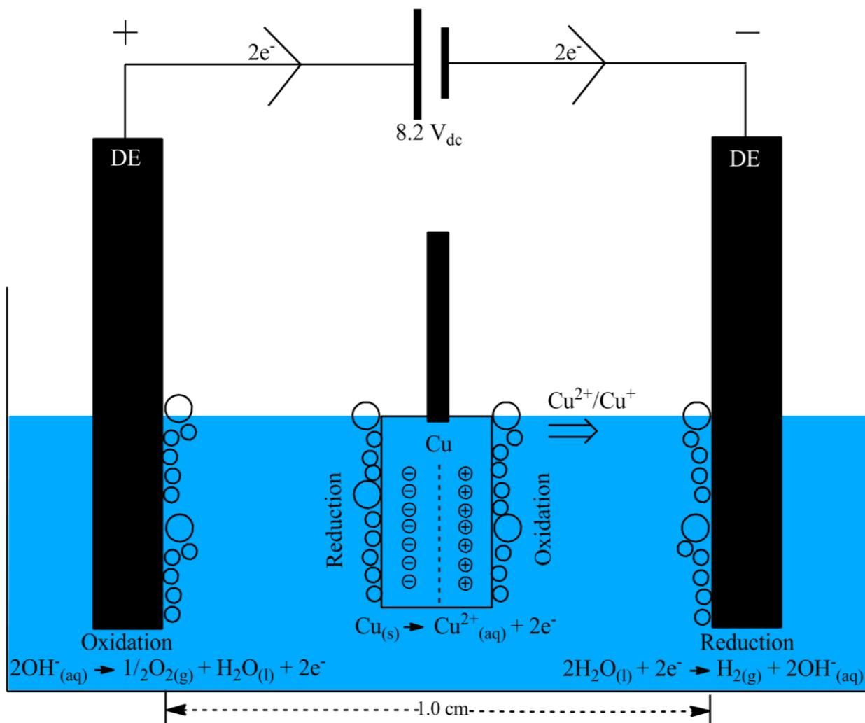
**Figure S1:** Schematic representing the bipolar electrochemical generation of copper ions for  $\text{Cu}_2\text{O}$  generation.
