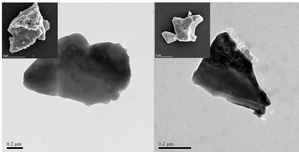
**Figure S15:** TEM and SEM (inserts) of commercial  $\text{Cu}_2\text{O}$ .
