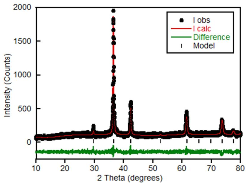
**Figure S4:** Refinement profile for the Rietveld analysis of room temperature XRD data that was collected for 4.5 V-1H and fitted to the model <sup>S1</sup>.
