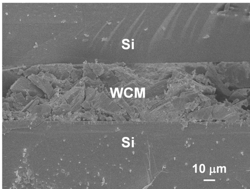
**Figure 2.** Cross-sectional scanning electron microscope image of a bonded interface (WCM concentration:  $1 \times 10^{-2}$  g/mL).
