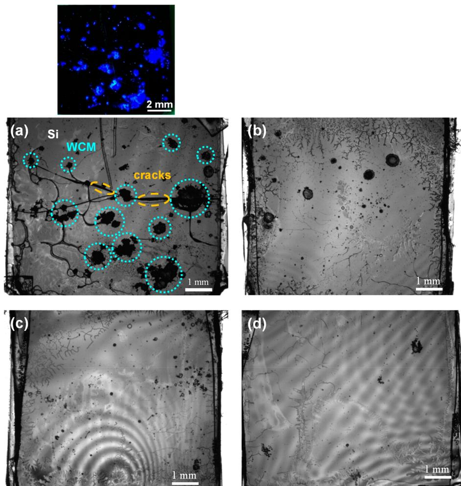
**Figure 4.** Infrared inner images of bonded interfaces (WCM concentration: (a)  $1 \times 10^{-2}$  g/mL, (b)  $5 \times 10^{-3}$  g/mL, (c)  $1 \times 10^{-3}$  g/mL, (d)  $1 \times 10^{-4}$  g/mL). The accompanying image (top) is an optical photograph of the debonded Si surface after the intentional debonding of the bonded sample of (a) under an ultraviolet lamp.
