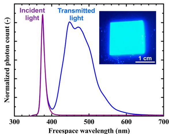
**Figure 6.** Transmission spectrum of the bonded samples with WCM and spectrum of the incident light. Inset: optical photograph of the bonded sample with WCM under an ultraviolet lamp.
