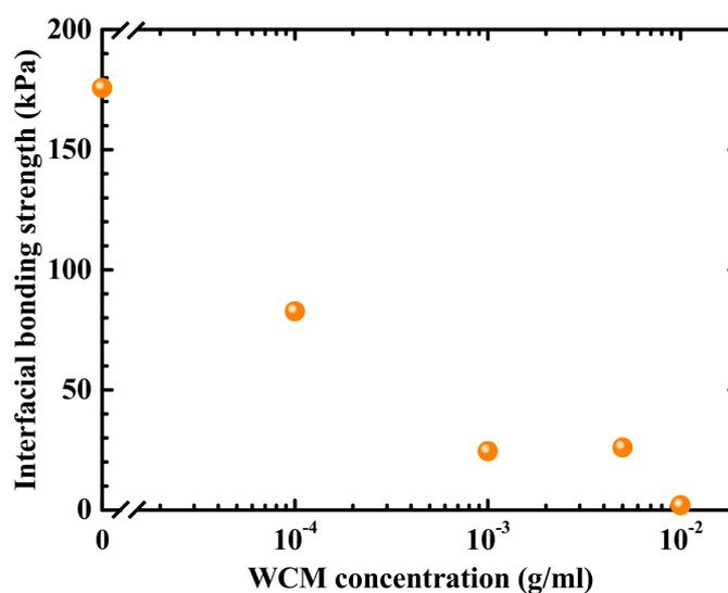
**Figure 3.** Interfacial bonding strength vs. WCM concentration.
