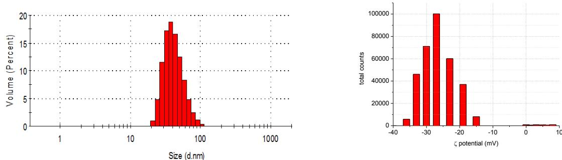
SI-Figure 4. DLS measurements of AgNPs-3MPS in presence of 1 ppm of  $Co^{2+}$ : a)  $\langle 2R_H \rangle = 76 \pm 9$  nm; b)  $\zeta$  potential =  $-22 \pm 15$  (mV)
