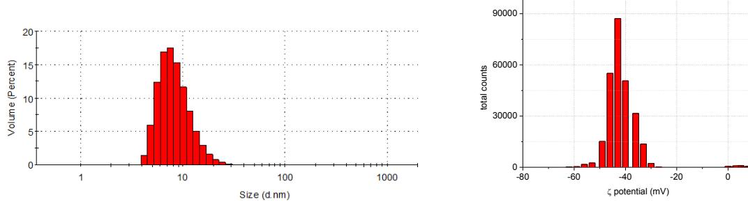
SI-Figure 3. DLS measurements of AgNPs-3MPS in presence of 1 ppm of  $Ni^{2+}$ : a)  $\langle 2R_H \rangle = 43 \pm 4$  nm; b)  $\zeta$  potential =  $-27 \pm 10$  (mV)
