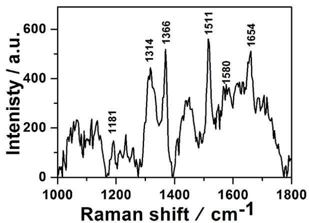
Figure S3. The normal Raman spectrum of 0.01 M R6G methanol solution.
