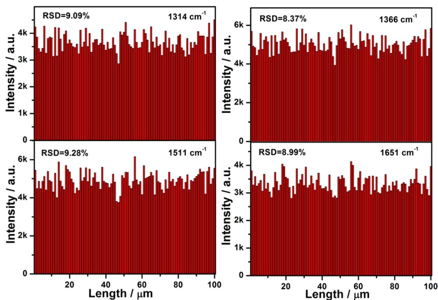
Figure S4. The intensities of the major peaks in the 100 SERS spectra of R6G solution ( $1 \times 10^{-8}$  M).
