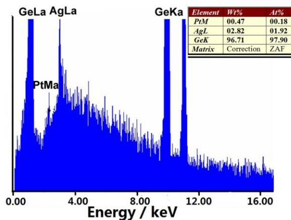
Figure S2. The EDS spectra of the the Ge wafer grown with Ag-Pt nanoparticles.
