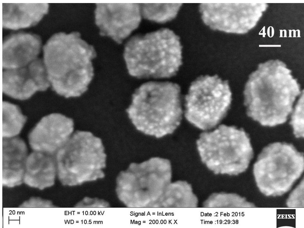
Figure S1. The high magnification SEM images of Ag-Pt nanoparticles grafted on the Ge wafer.
