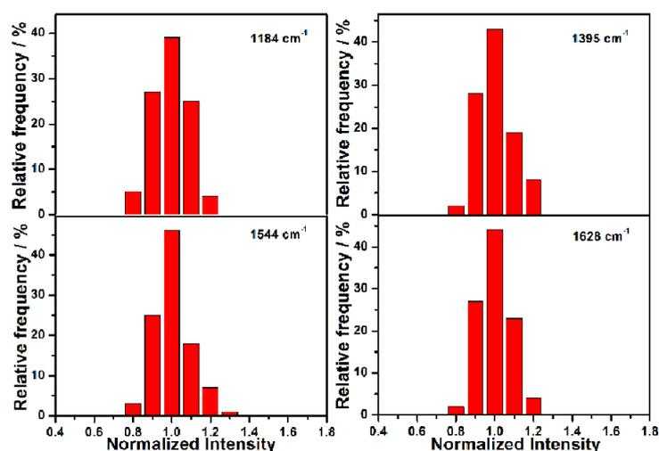
**Figure S7.** Histograms of normalized Raman intensities of CV ( $1 \times 10^{-7}$  M) on Ag-Pt NPs/Ge SERS substrate.
