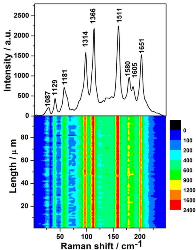
Figure S8. (Upper) the SERS spectrum of  $1 \times 10^{-8}$  M R6G solution on Ag-Pt NPs/Ge SERS substrate after a one-year storage in atmospheres at room temperature. (Lower) the SERS contour from line mapping of 100 spots.
