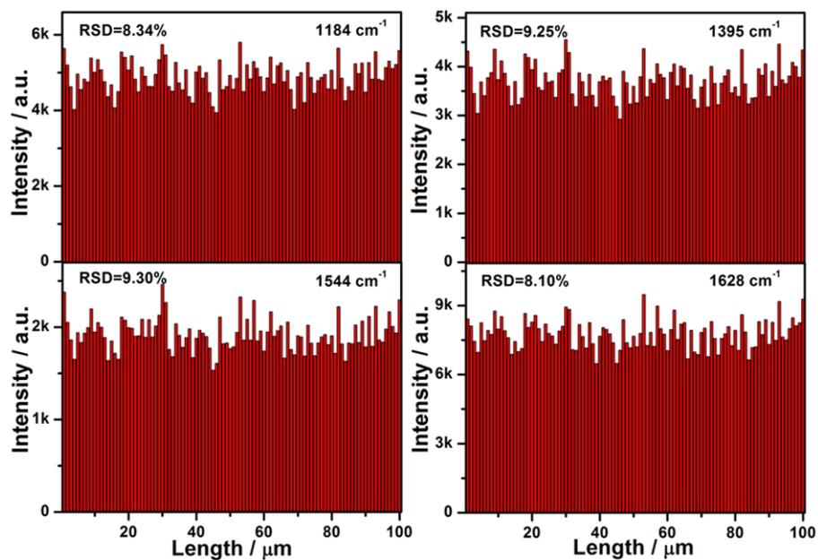
**Figure S6.** The intensities of the major peaks in the 100 SERS spectra of  $1 \times 10^{-7}$  M CV solution.
