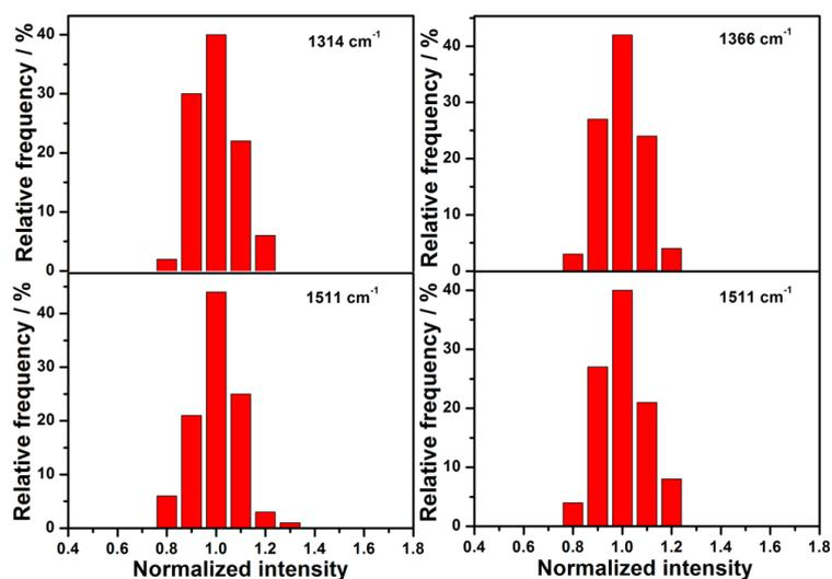
Figure S5. Histograms of normalized Raman intensities of R6G ( $1 \times 10^{-8}$  M) on Ag-Pt NPs/Ge SERS substrate.
