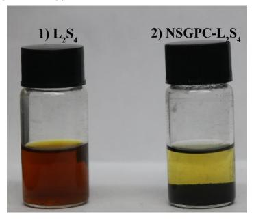
Figure S3. Digital photograph of Li<sub>2</sub>S<sub>4</sub> solution and after adding NSGPC.
