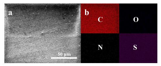
**Figure S7.** SEM image (a) and corresponding elemental mappings (b) of the back of NSGPC-coated separator (facing to the Li anode) after 100 cycles at 0.2 C.
