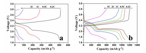
**Figure S4.** Discharge/charge voltage profiles of the Li-S batteries with (a) PP and (b) NSGPC-coated separators at various current rates. The sulfur mass loading of the simple cathodes was about 1.3 mg cm<sup>-2</sup>.
