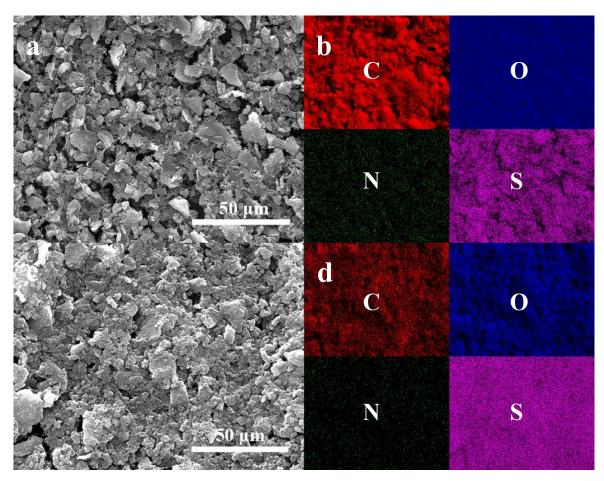
**Figure S6.** SEM images and corresponding elemental mappings of NSGPC-coated separator (a,b) before cycles and (c,d) after 100 cycles at 0.2 C.
