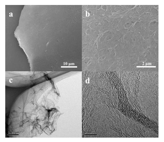
Figure S1. SEM images of pure G (a-b), TEM and HRTEM images of pure G (c-d).
