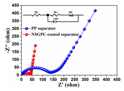
**Figure S8.** EIS curves of the fresh Li-S batteries with PP and NSGPC- coated separators, and the inset is equivalent circuit model.
