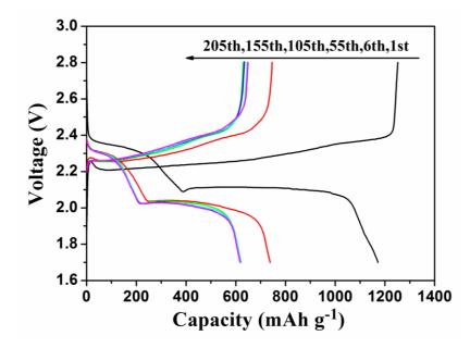
**Figure S5.** Discharge/charge voltage profiles of the Li-S batteries with NSGPC-coated separator at various cycles. The sulfur mass loading of the simple cathodes was about 3.4 mg cm<sup>-2</sup>.
