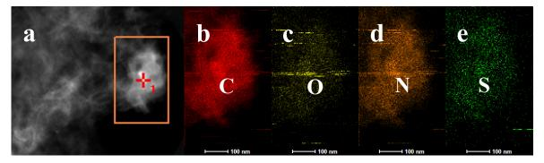
**Figure S2.** STEM image of NSGPC (a), corresponding elemental maps of carbon (b), oxygen (c), nitrogen (d), and sulfur (e).
