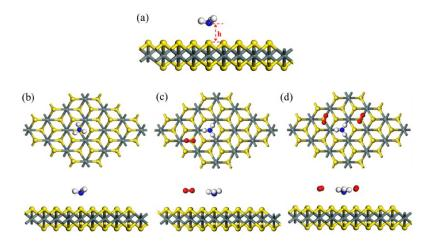
**Figure 3.** (a) Optimized  $6 \times 6$  supercell of SnS<sub>2</sub> (h represents the closest distance between NH<sub>3</sub> and the SnS<sub>2</sub> surface), (**b**–**d**) top views and side views of the SnS<sub>2</sub> surface with no O<sub>2</sub>, one O<sub>2</sub>, and two pre-adsorbed O<sub>2</sub> molecules, pre-adsorption. Red, silver, blue, yellow, and cyan balls represent O, H, N, S, and Sn atoms, respectively (reproduced from [29], with permission from ELSEVIER, 2018).
