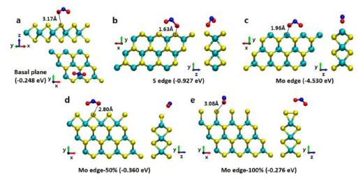
**Figure 4.** Schematics of NO<sub>2</sub> molecules adsorbed on (**a**) the basal plane, (**b**) S edge, (**c**) Mo edge, (**d**) Mo edge-50%, (**e**) and Mo-edge-100%. Cyan, red, yellow, and blue spheres represent molybdenum, oxygen, sulfur, and nitrogen, respectively (reproduced from [60], with permission from American Chemical Society, 2018).
