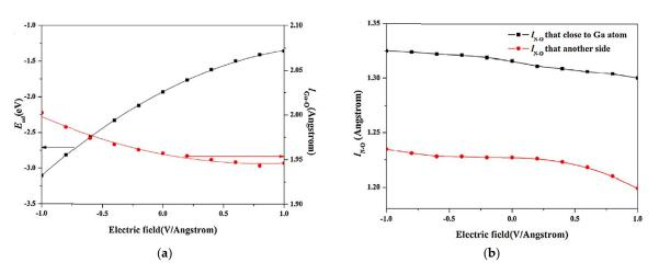
**Figure 6.** Variation of (**a**) adsorption energy ( $E_{ad}$ ) and bond length of Ga–O ( $l_{Ga-O}$ ), (**b**) charge transfer on NO<sub>2</sub> molecule under various electric field (reproduced from [85], with permission from ELSEVIER, 2018).
