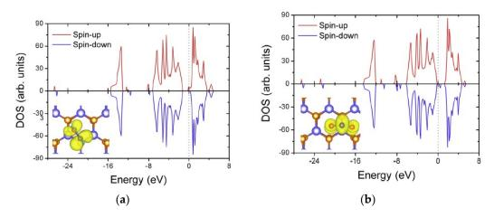
**Figure 2.** Spin-polarized density of states (DOS) of (**a**) NO and (**b**) NO<sub>2</sub> adsorbed on MoS<sub>2</sub> (reproduced from [22], with permission from ELSEVIER, 2018).
