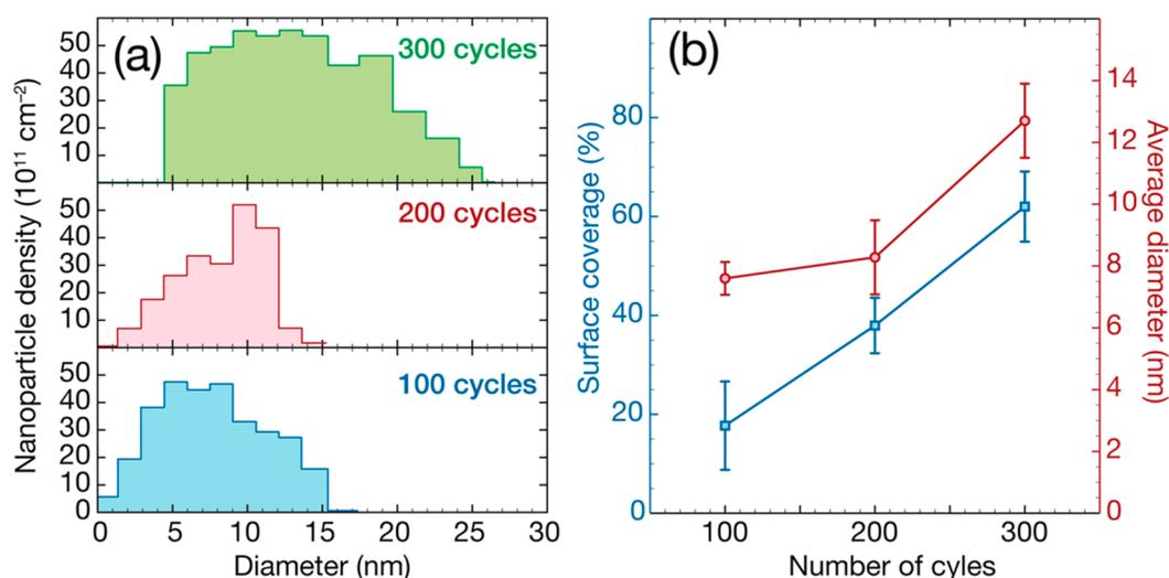
**Figure 2.** (a) Nanoparticle (NP) size distribution and (b) average diameter and surface density evolution of the Pd NPs on BN surfaces after 100, 200 and 300 ALD cycles (estimated). The data analysis is based on the TEM images presented in Figure 1.
