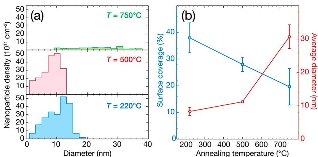
**Figure 5.** (a) Nanoparticle size distribution and (b) average diameter and surface coverage evolution of the Pd NPs on BN surfaces, as prepared at 220 °C and after thermal treatments at 500 and 750 °C for 3 h. The data analysis is based on the TEM images presented in Figure 4.
