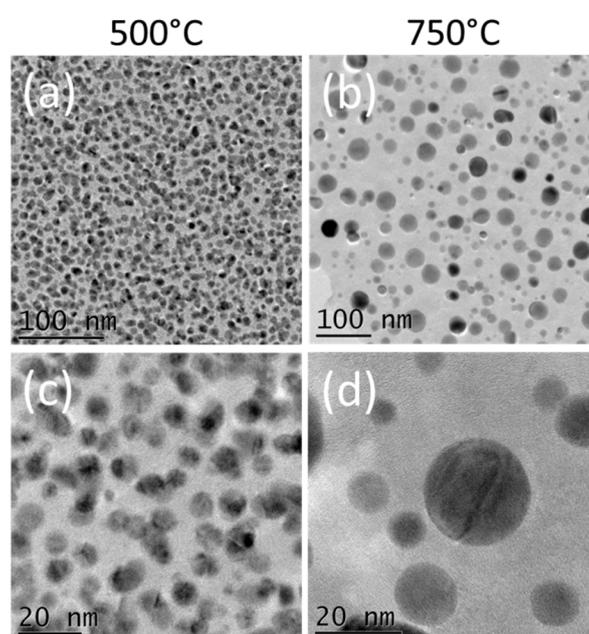
**Figure 4.** TEM images of Pd NPs on BN surfaces prepared by applying 200 cycles of the Pd ALD process, after heating treatments at (a,c) 500 °C and (b,d) 750 °C for 3 h. The substrates used were Si<sub>3</sub>N<sub>4</sub> TEM window grids covered with 15 nm of BN.
