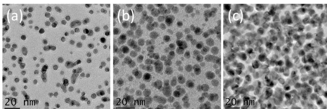
**Figure 1.** Transmission electron microscopy (TEM) images of boron nitride (BN) surfaces after (a) 100, (b) 200, and (c) 300 cycles of the Pd atomic layer deposition (ALD) process. The substrates used were  $\text{Si}_3\text{N}_4$  TEM windows covered with 15 nm of BN.
