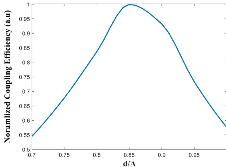
**Figure 2.** Normalized coupling efficiency as a function of the geometrical parameters of the multicore photonic crystal fiber (PCF) ( $d/\Lambda$ ) for the operating wavelengths.
