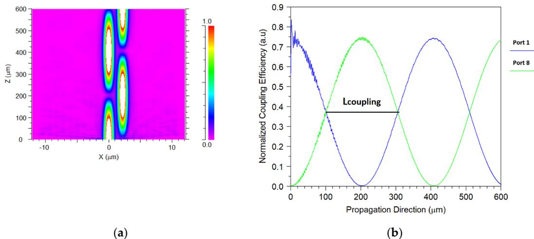
**Figure 3.** Energy transfer between core 1 and core 8 for the 1565-nm wavelength. (a). Intensity profile. (b). Normalized coupling efficiency as a function of the propagation direction.
