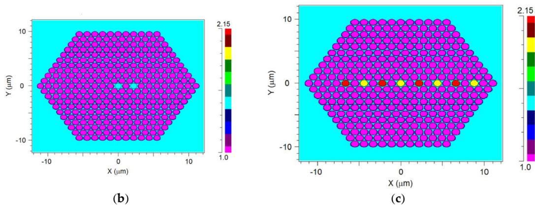
**Figure 1.** Refractive index profile of the  $1 \times 8$  wavelength demux: (a) XZ plane at  $y = 0$  cm. (b) XY plane at  $z = 0$  cm. (c) XY plane at  $z = 5$  cm.
