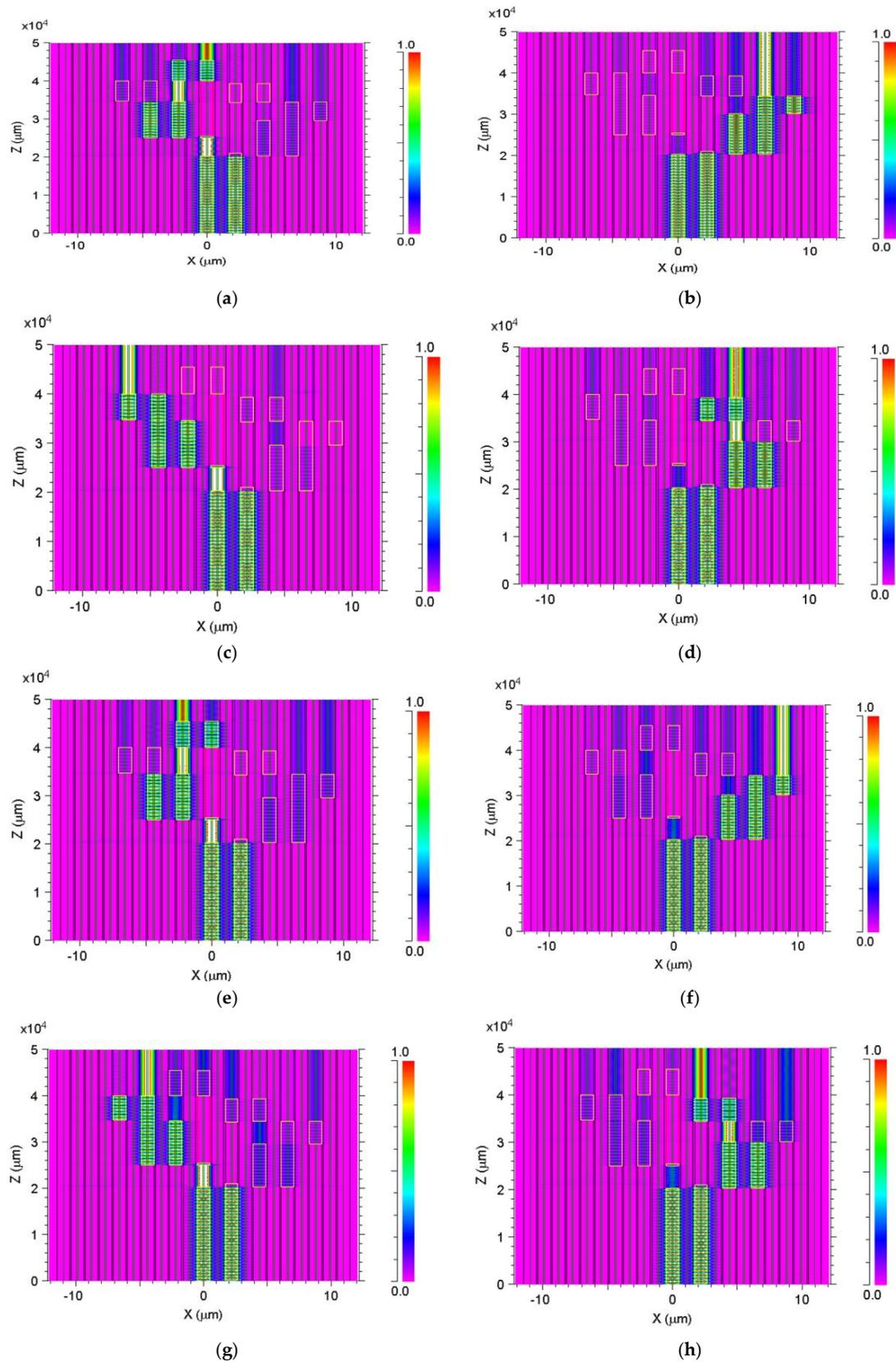
**Figure 4.** Intensity profile of the  $1 \times 8$  multimode interference (MMI) wavelength demultiplexer: (a)  $\lambda_1 = 1530$  nm (port 1). (b)  $\lambda_2 = 1535$  nm (port 2). (c)  $\lambda_3 = 1540$  nm (port 3). (d)  $\lambda_4 = 1545$  nm (port 4). (e).  $\lambda_5 = 1550$  nm (port 5). (f)  $\lambda_6 = 1555$  nm (port 6). (g)  $\lambda_7 = 1560$  nm (port 7). and (h)  $\lambda_8 = 1565$  nm (port 8).
