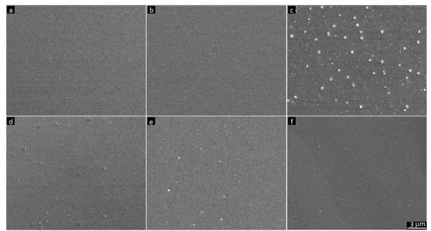
**Figure S1.** AgCl formation on top of the AgNP films (SEM images). AgCl formation occurred when the AgNP films were printed on paper coatings containing a sufficient concentration of Cl. a) HP10 reference, b) HP22 reference, c) HP22 reference (pretreated with 0.3 M KCl), d) HP10 active, e) HP22 active, and f) HP22 active (ethanol+EG ink) papers.
