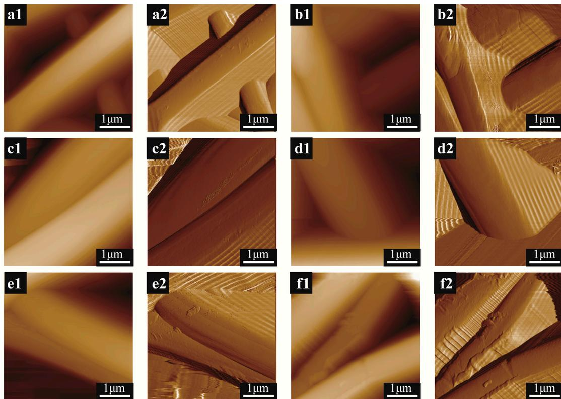
**Figure 4.** Height (a1,b1,c1,d1,e1,f1) and Peak Force Error (a2,b2,c2,d2,e2,f2) images of PLA nanofibers with different mineralization time: (a1,a2) 0-day; (b1,b2) 1-day; (c1,c2) 3-day; (d1,d2) 5-day; (e1,e2) 7-day; (f1,f2) 21-day.
